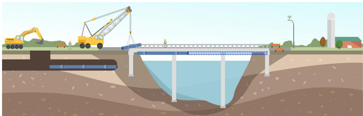
Figure 6-6: Suspended Construction Methodology from a Bridge
