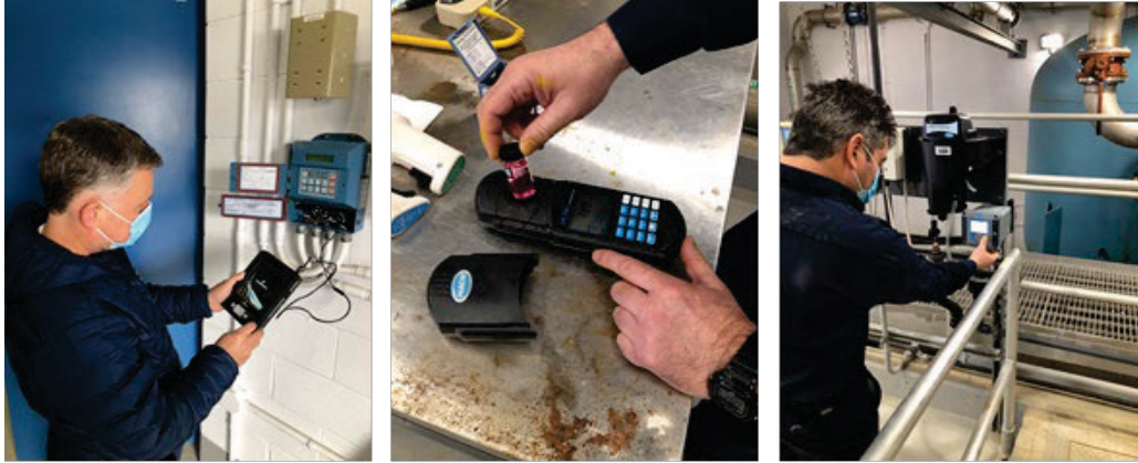
Figure 15. Staff calibrating level transmitter and verifying handheld chlorine analyzer and online turbidity analyzer
