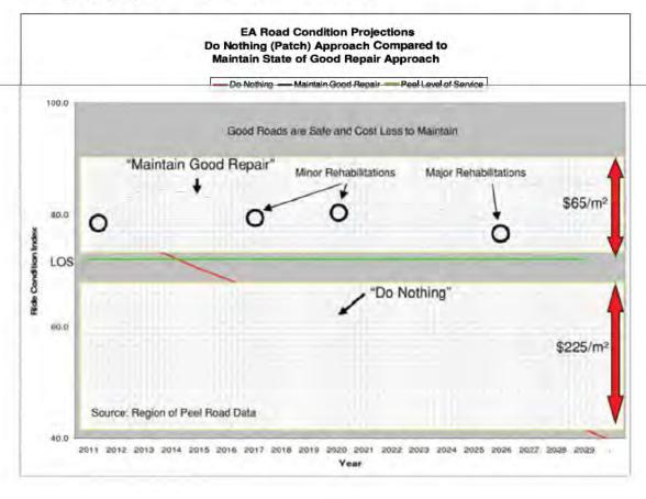
The analysis completed to date for the EA verifies the base and pavement conditions of the roads have cracking, heaving and drainage deficiencies. These conditions do not lend themselves to simple band aid patch solutions and reconstruction will be the more cost effective approach in the long term.
