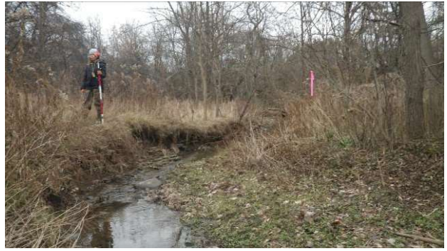
XS 10: View facing downstream. Note bank erosion along outside meander bend (left bank). Right bank has gradual slope.
