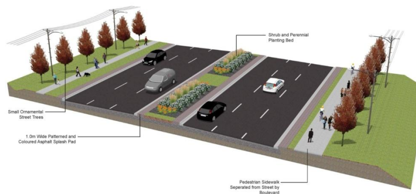
Figure 6.1.2 – Landscape Cross Section – Ultimate 6 Lanes With Median
