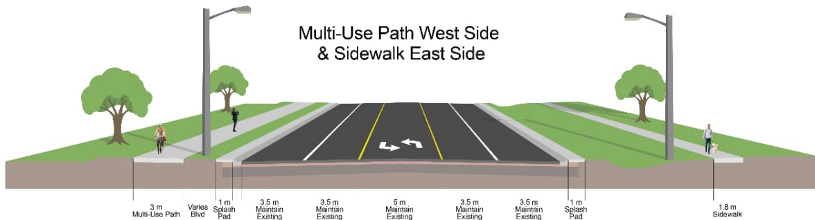
Figure 6.19 – AT Alternative 7 West MUP and East Sidewalk
