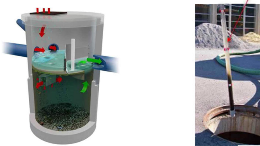
Figure 6.7 – SWM Alternative 6 Oil and Grit Separators
