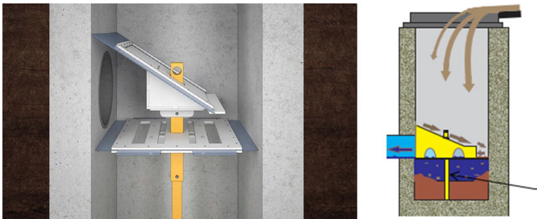
Figure 6.11 – SWM Alternative 10 Catchbasin Shields
