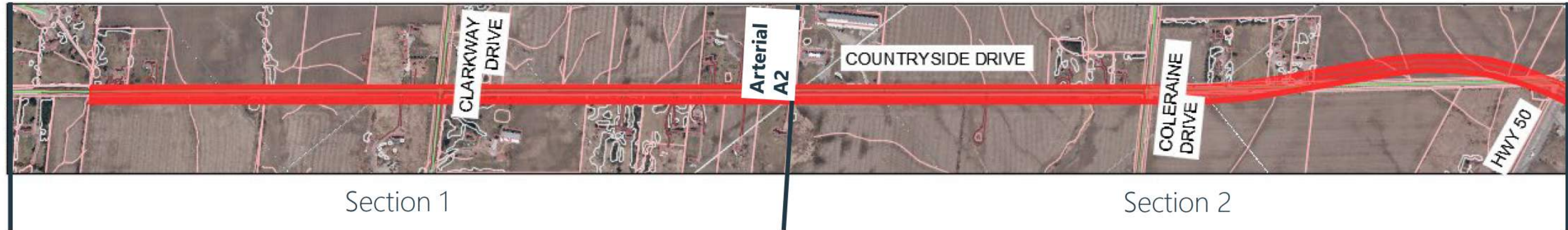
Countryside Drive (Alternative 3 – Widen to the South of Existing Right-of-Way and Curve Through Hwy 50 Intersection)
