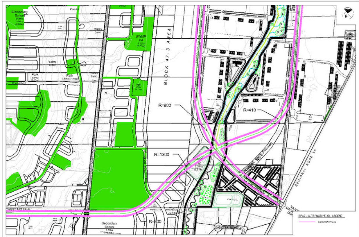
Figure 5-6: Recommended Arterial Road Configuration for SPA 2
