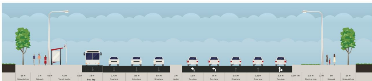
Figure 6-3: Arterial A2 – Recommended Cross-Section, Intersection
