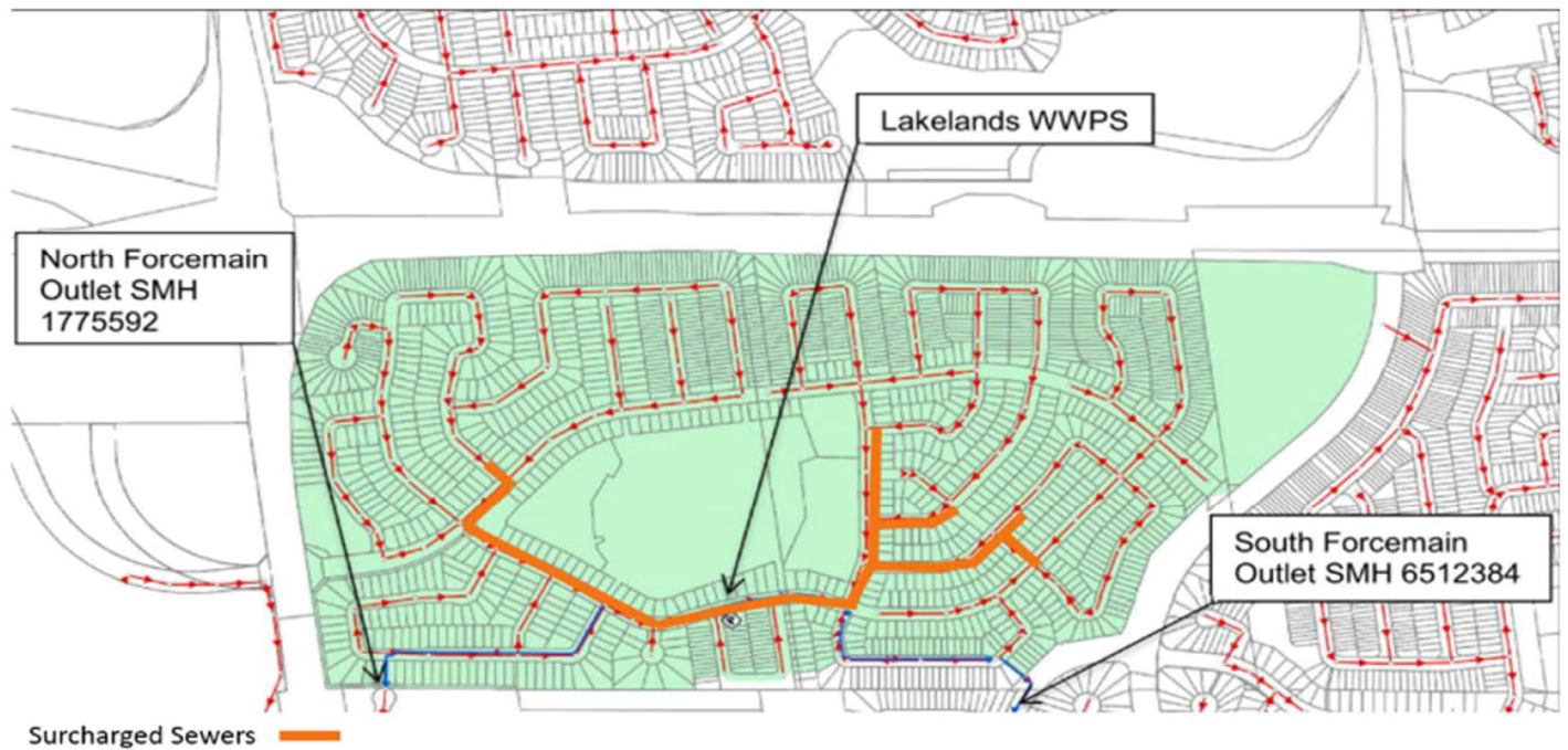
Figure 5-2: Surcharged Sewers after 2-Hour Shutdown at Lakelands WWPS
