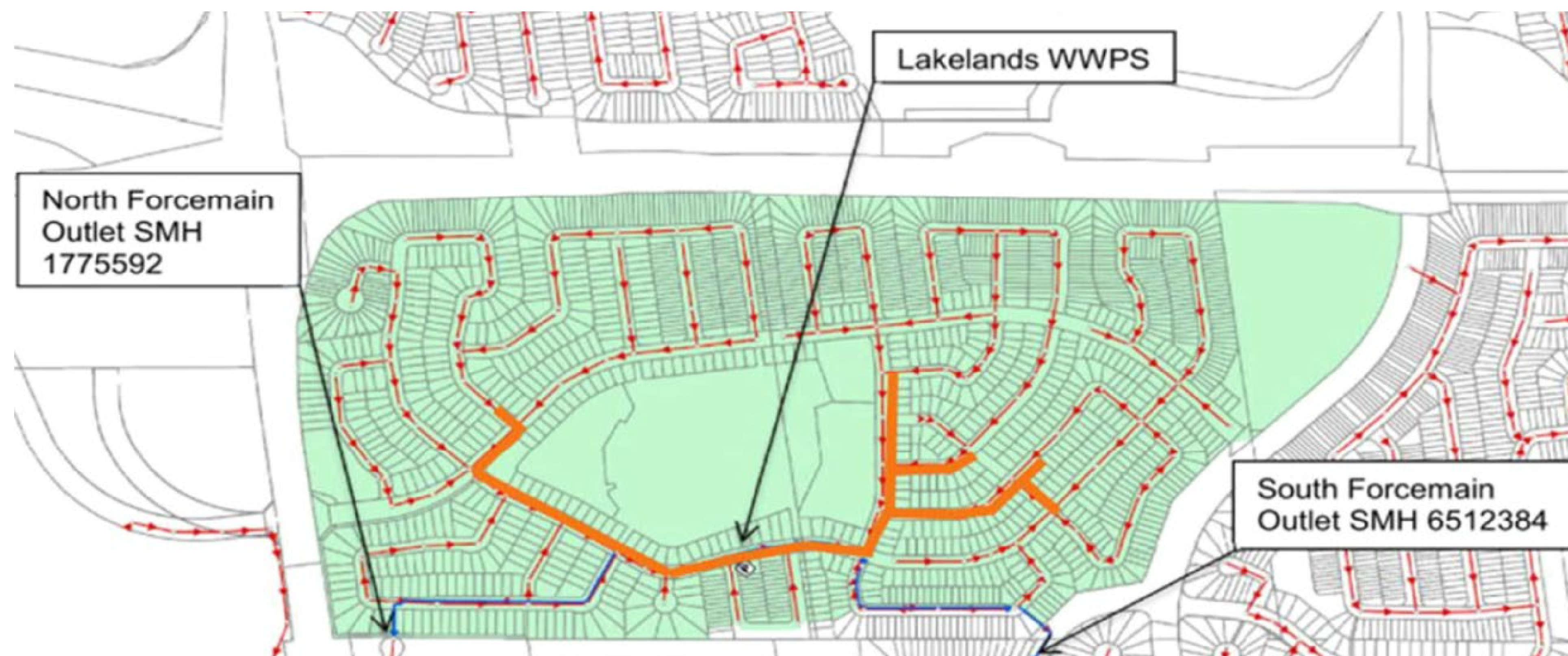
Surcharged Sewers after 2-Hour Shutdown at Lakelands WWPS
