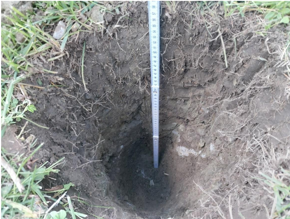
Image 10: Representative test pit demonstrating disturbed stratigraphy.
