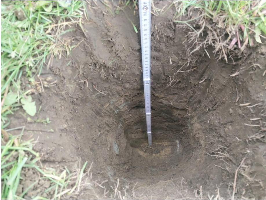
Image 9: Representative test pit demonstrating disturbed stratigraphy.
