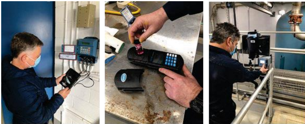
Figure 9. Staff calibrating level transmitter and verifying handheld chlorine analyzer and online turbidity analyzer
