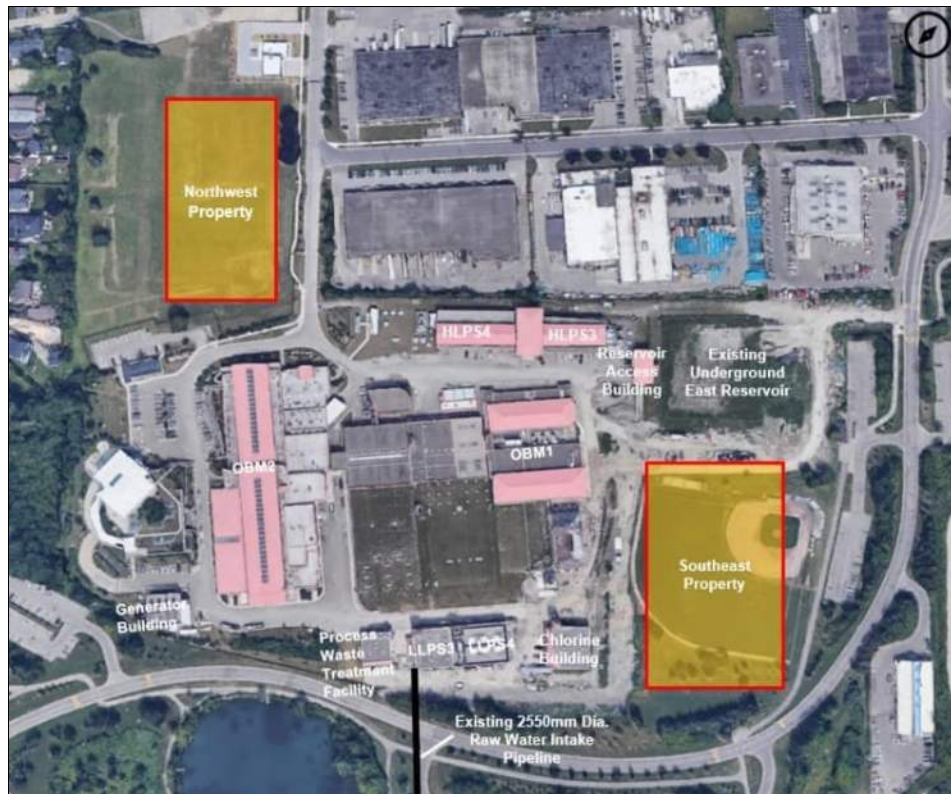
Figure 8-1: Short-Listed Alternative Solutions (onsite) for Reservoir Expansion
