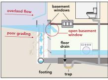
graded away basement windows from home trom home wall basement wall basement floor wastwater
