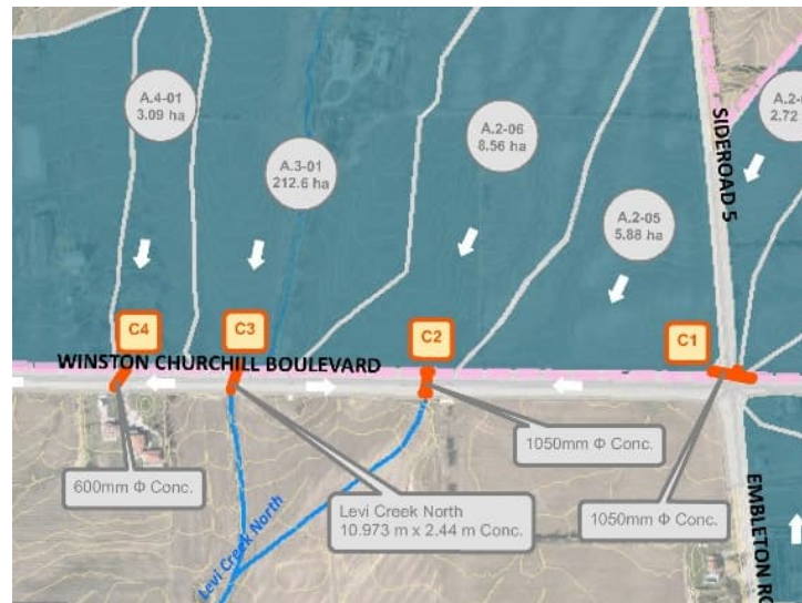
Figure 6-3: Culvert 3 Location – Levi Creek North
