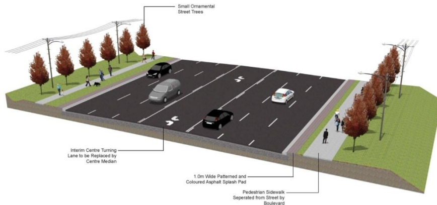
Figure 6.1.1 – Landscape Cross Section – Ultimate 6 Lanes Without Median
