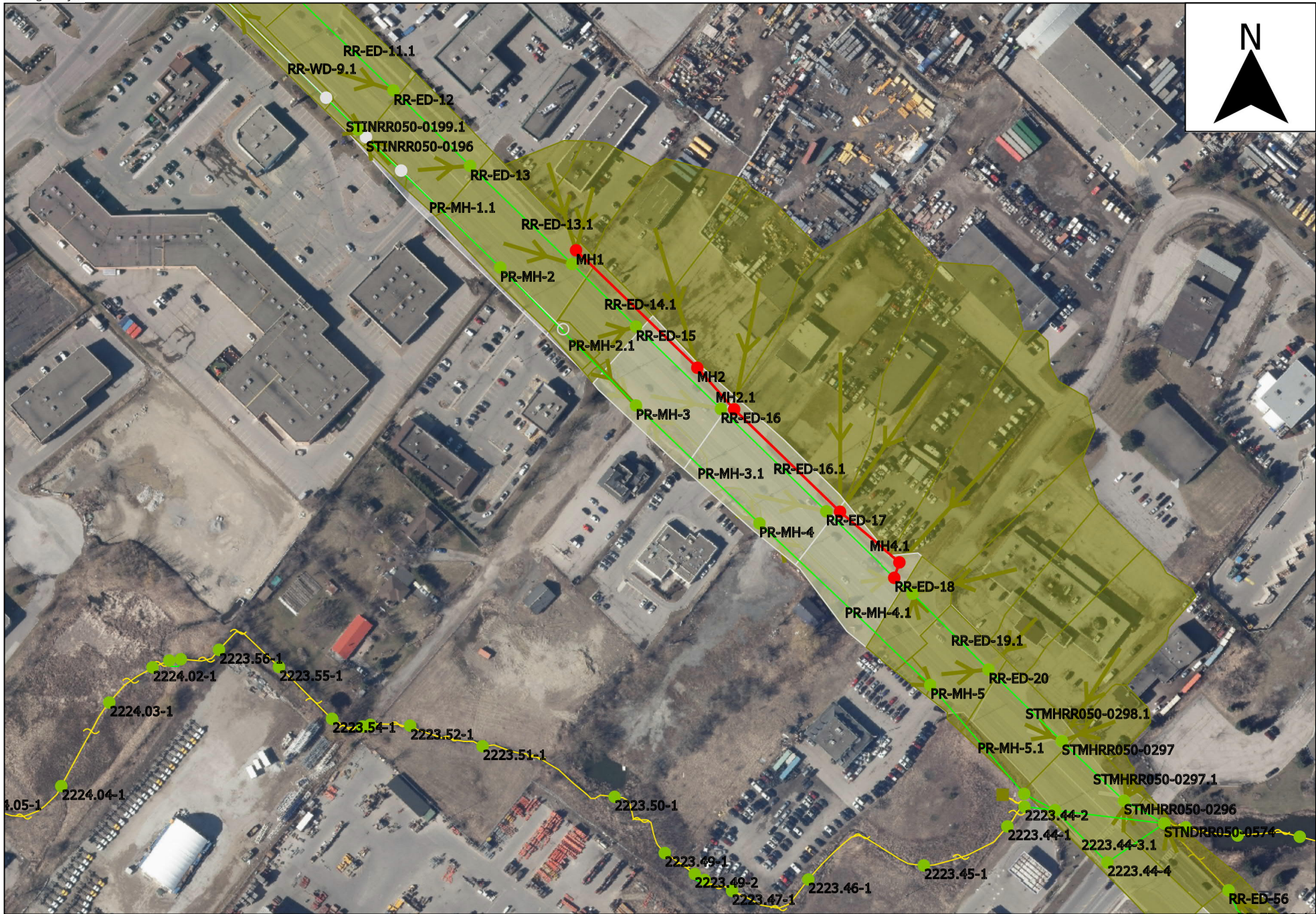
PROPOSED CONDITION - 100-YEAR - EAST SIDE PLAN 2-1 (PROPOSED STORM SEWERS UNDERNEATH THE PROPOSED SIDEWALK)
