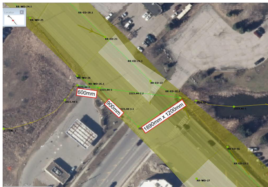
Figure 5.1: George Bolton Parkway and RR50 Intersection Culverts
