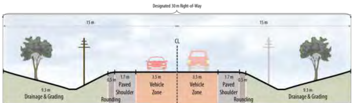
Figure 79: Option 3 - 11.4 m Platform Rural Option Considered for Bush Street
