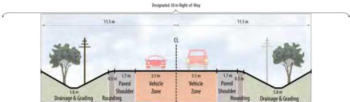
Figure 58: Option 3 - 11.4 m Platform Rural Option Considered for Olde Base Line Road
