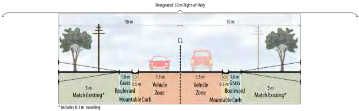
Figure 60: Option 6 - 10 m Platform Semi-Rural Option Considered for Olde Base Line Road
