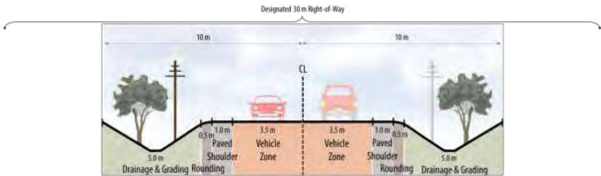
Figure 50: Option 2 - 10 m Platform Rural Option Considered for Winston Churchill Blvd
