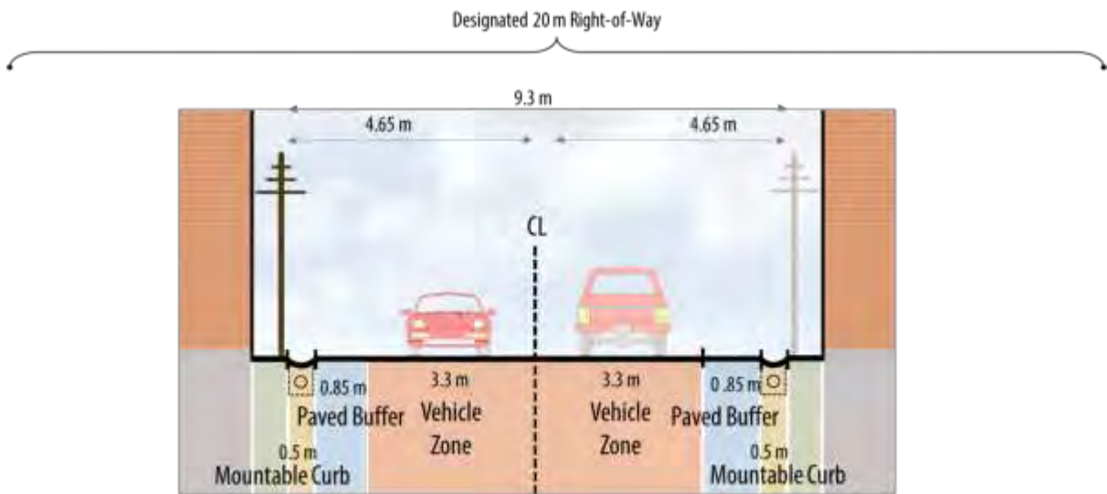
Figure 71: Option 4 - 9.3 m Platform Semi-Rural Option with Paved Buffer Considered for Village
