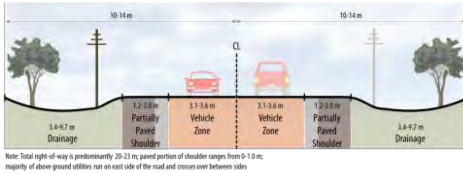
Figure 49: Option 1 - Do Nothing – Existing Conditions on Winston Churchill Blvd
