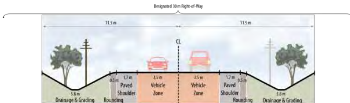
Figure 62: 11.4 m Platform Rural Cross-Section for Olde Base Line Road
