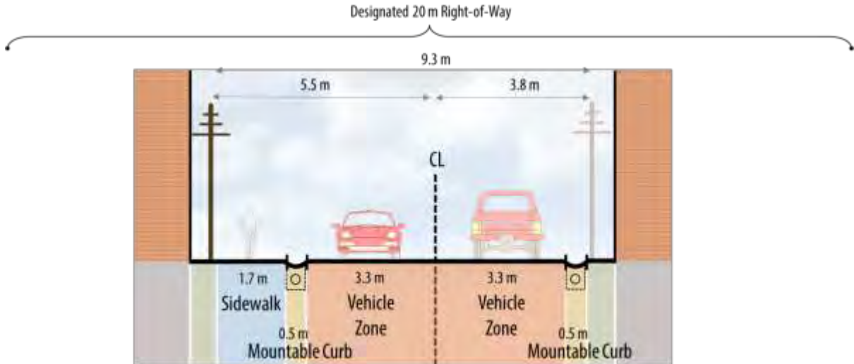
Figure 74: 9.3 m Platform Semi-Rural Cross-Section with Sidewalk for Belfountain Village (Shaws Creek Rd. to Mississauga Rd. / Old Main St.)
