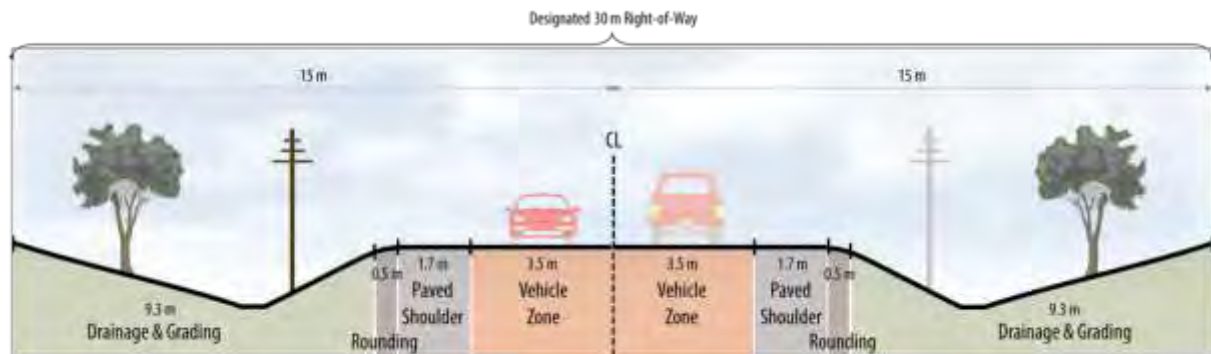
Figure 80: 11.4 m Platform Rural Cross-Section for Bush Street
