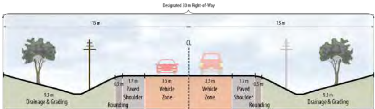
Figure 65: Option 3 - 11.4 m Platform Rural Option Considered for Mississauga Rd. / Old Main St.
