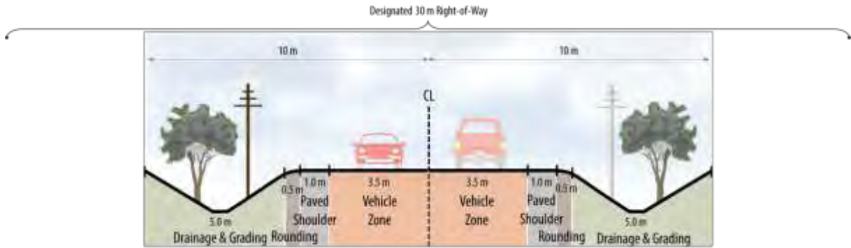
Figure 57: Option 2 - 10 m Platform Rural Option Considered for Olde Base Line Road
