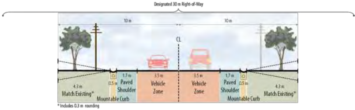
Figure 66: Option 4 - 11.4 m Platform Semi-Rural Option Considered for Mississauga Rd. / Old Main St.
