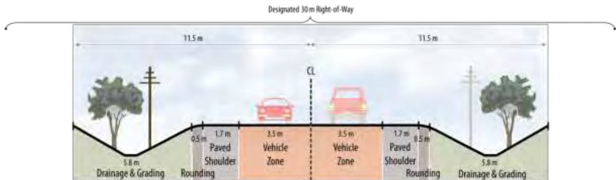
Figure 55: 11.4 m Platform Rural Cross-Section for Winston Churchill Boulevard
