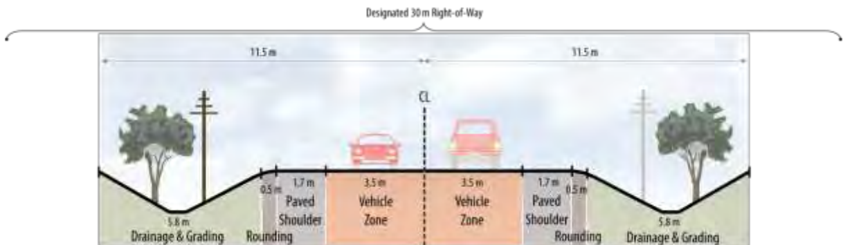
Figure 51: Option 3 -11.4 m Platform Rural Option Considered for Winston Churchill Blvd
