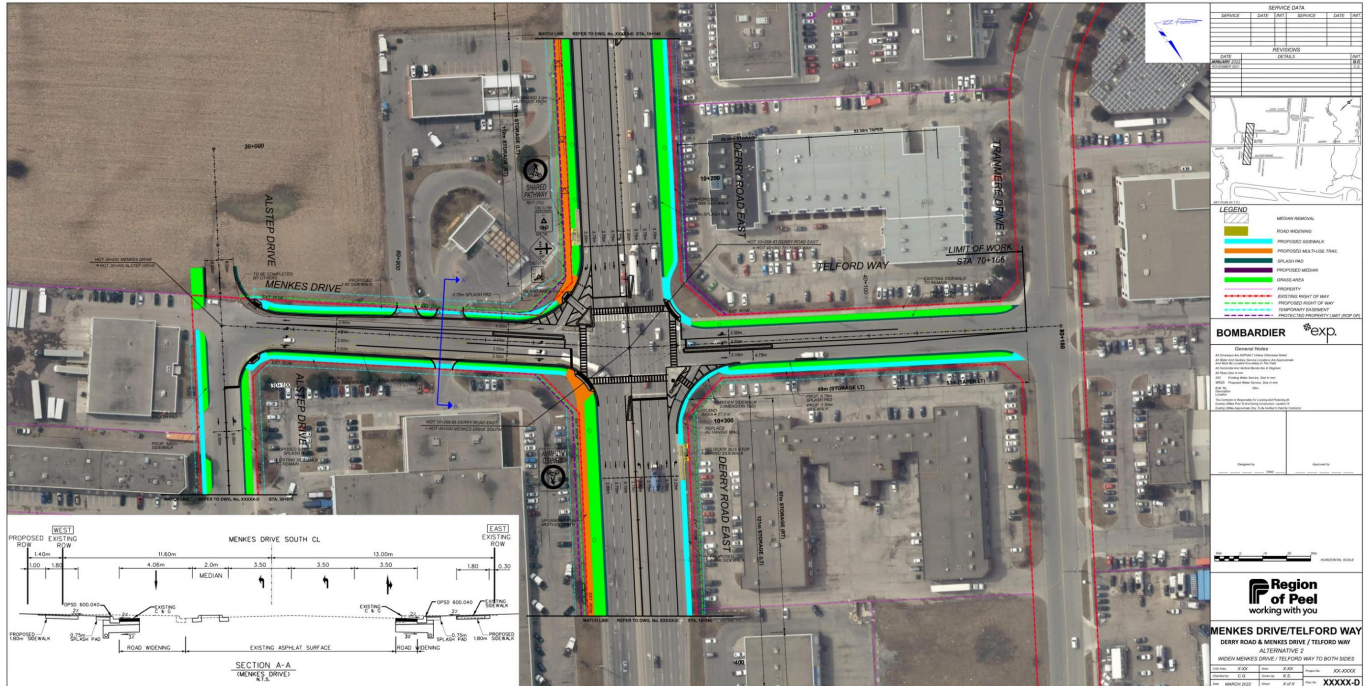
Figure 23: Derry Road East & Menkes Drive/Telford Way Preferred Alternative Design Concept
