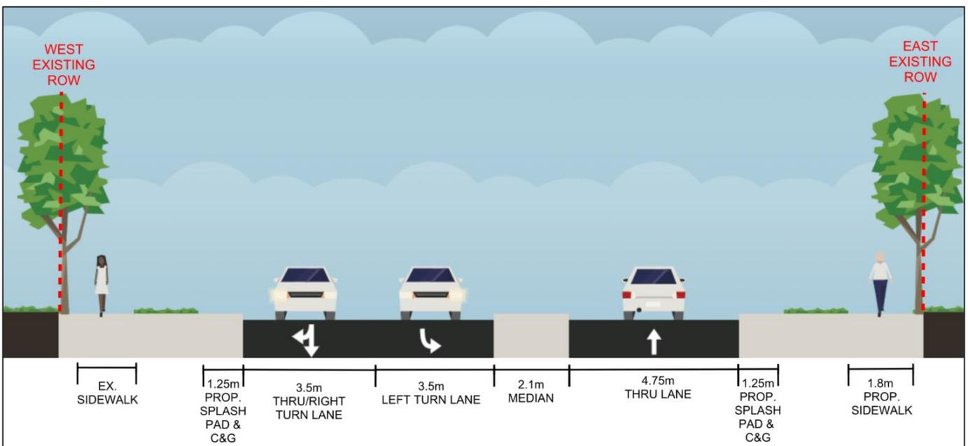
Figure 18: Menkes Drive/Telford Way Typical Cross-Section on Telford Way
