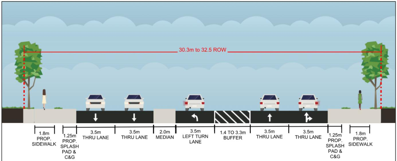
Figure 19: Typical Cross-Section of for Bramalea Road, South of Derry Road (facing north)
