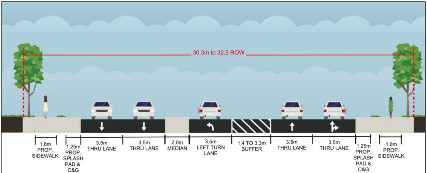
Figure 17: Menkes Drive/Telford Way Typical Cross Section on Menkes Drive (facing north)
