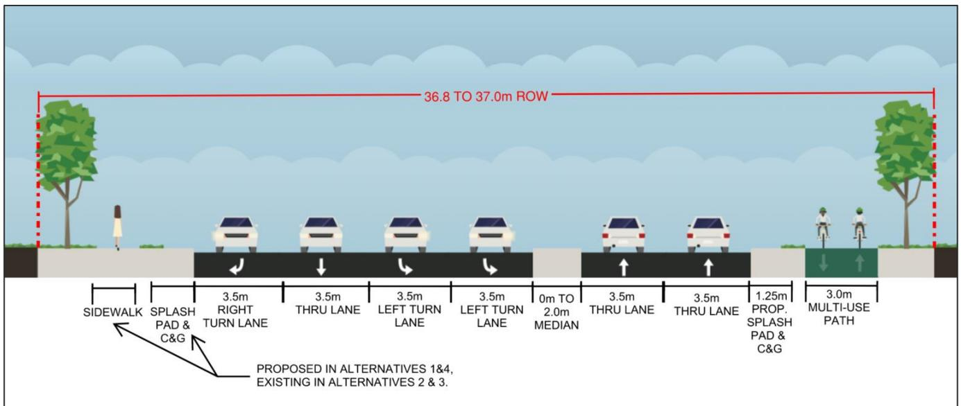
Figure 20: Typical Cross-Section for Bramalea Road, North of Derry Road (facing north)
