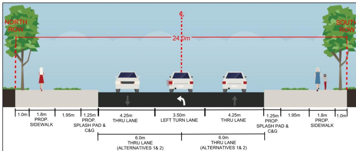
Figure 16: Alstep Drive Alternatives Typical Cross-Section <sup>15</sup>
