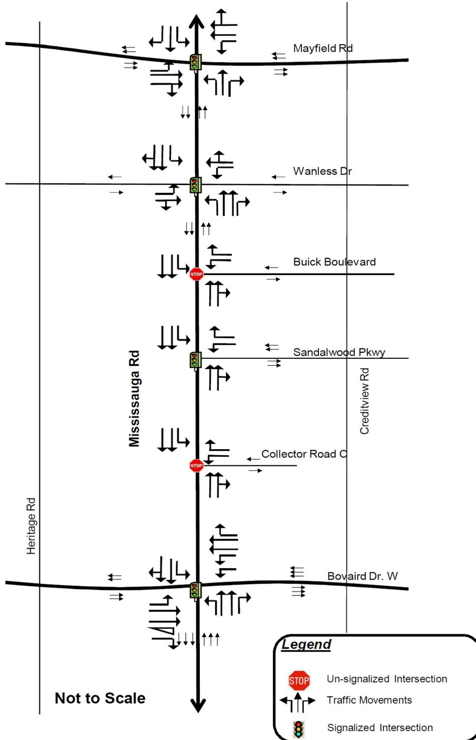
**Table 11** shows the corridor level of service with road improvement. With four lanes on Mississauga Road between Bovaird Drive West and Mayfield Road, the corridor is expected to operate with residual capacity during both the AM and PM peak period.
