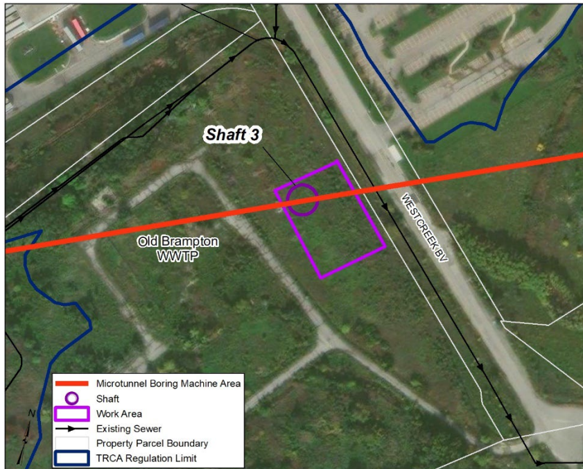
Figure 7-19. Shaft 3 Compound Area
