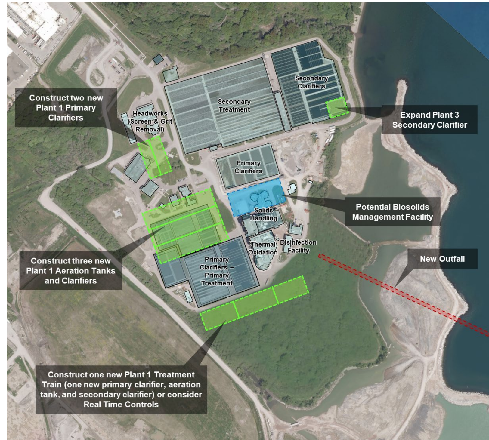
Expand G.E. Booth WWTP from 500 MLD to 550 MLD
