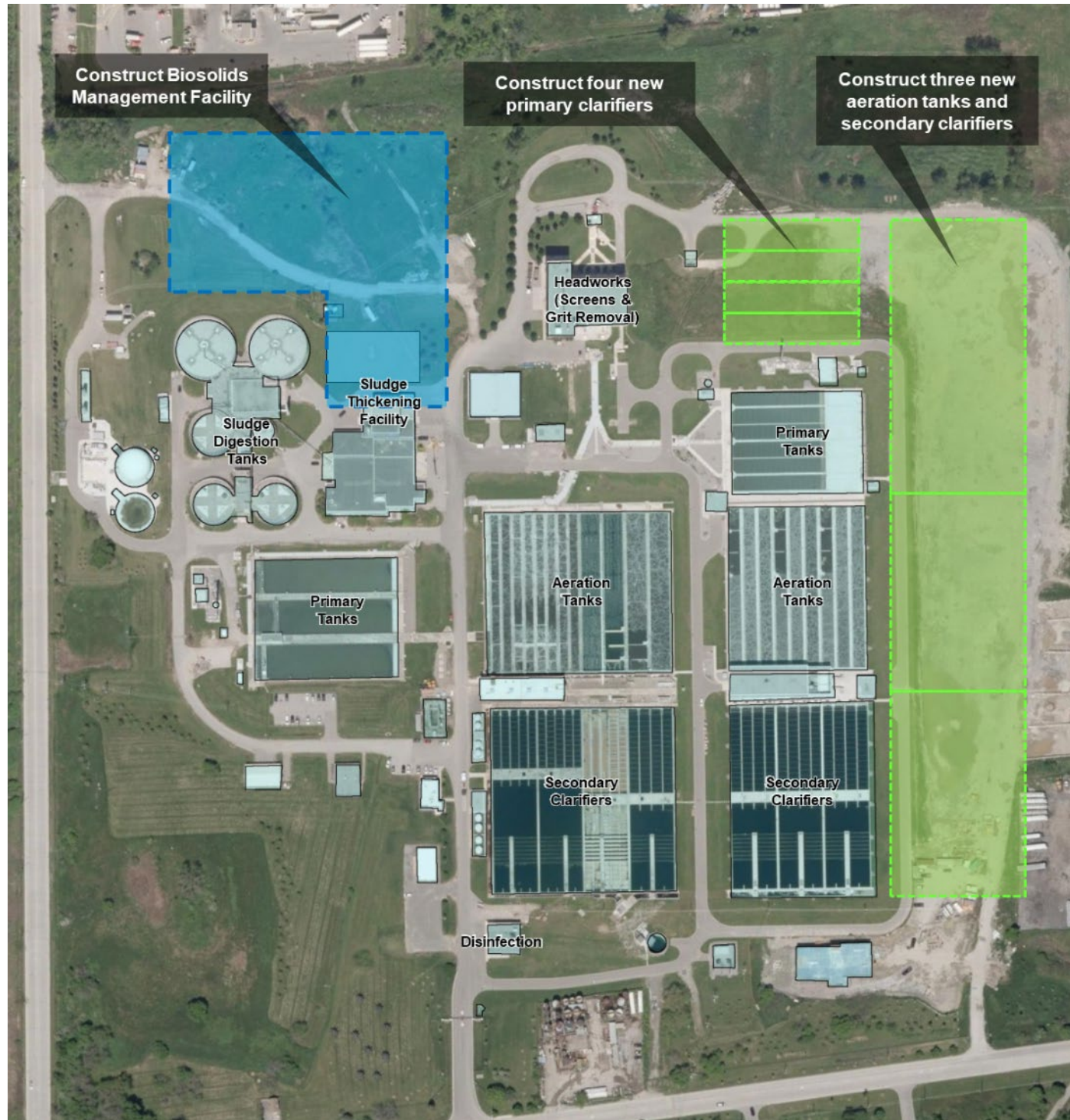
Expand Clarkson WWTP from 350 MLD to 500 MLD
