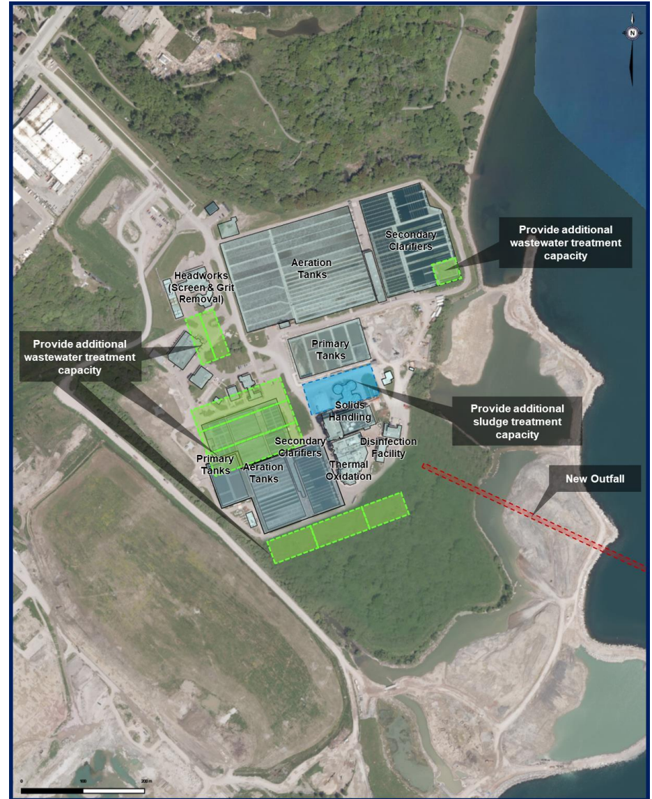
G.E. Booth Wastewater Treatment
