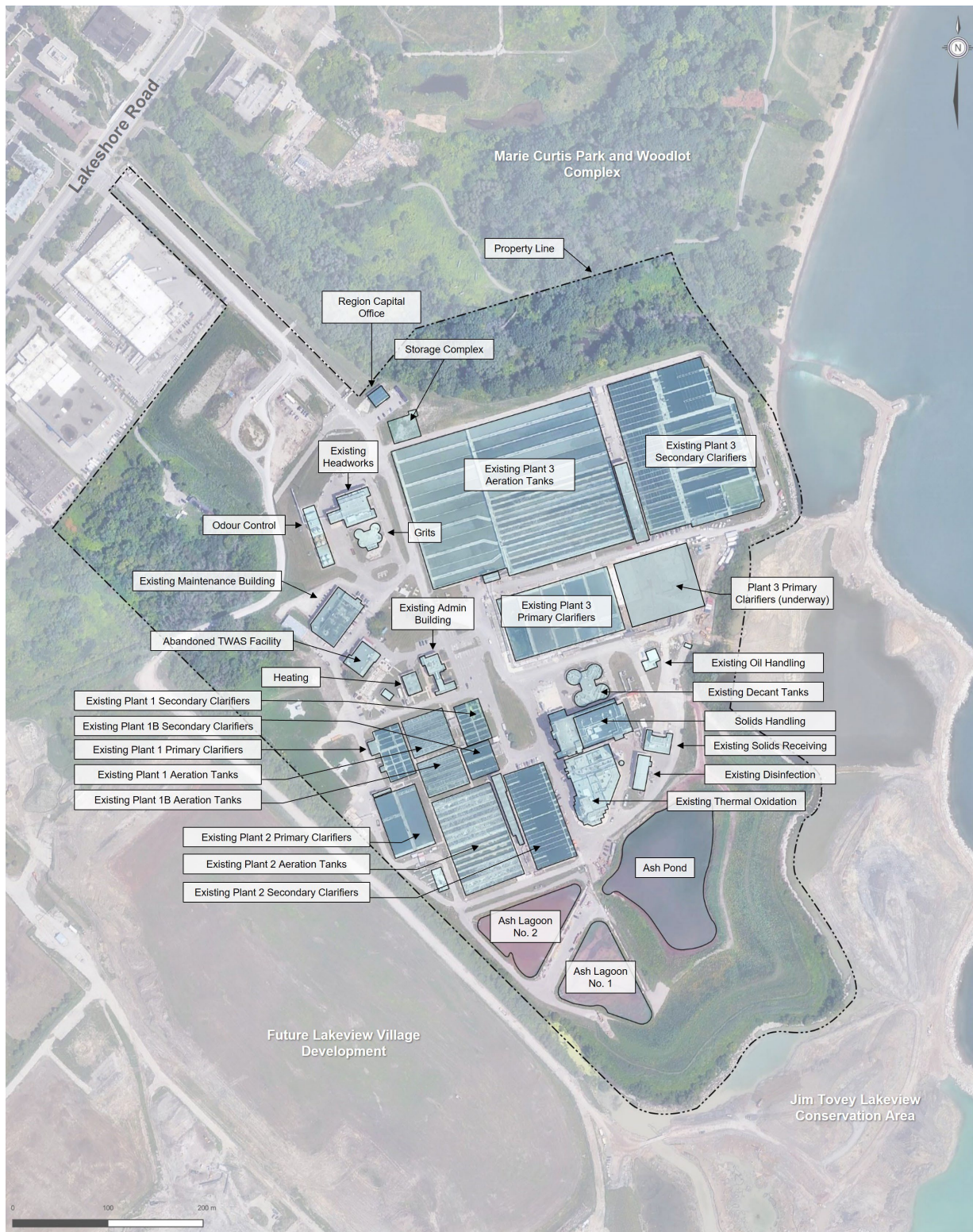
Figure 5-6: G.E. Booth WRRF Existing Plant Facilities
