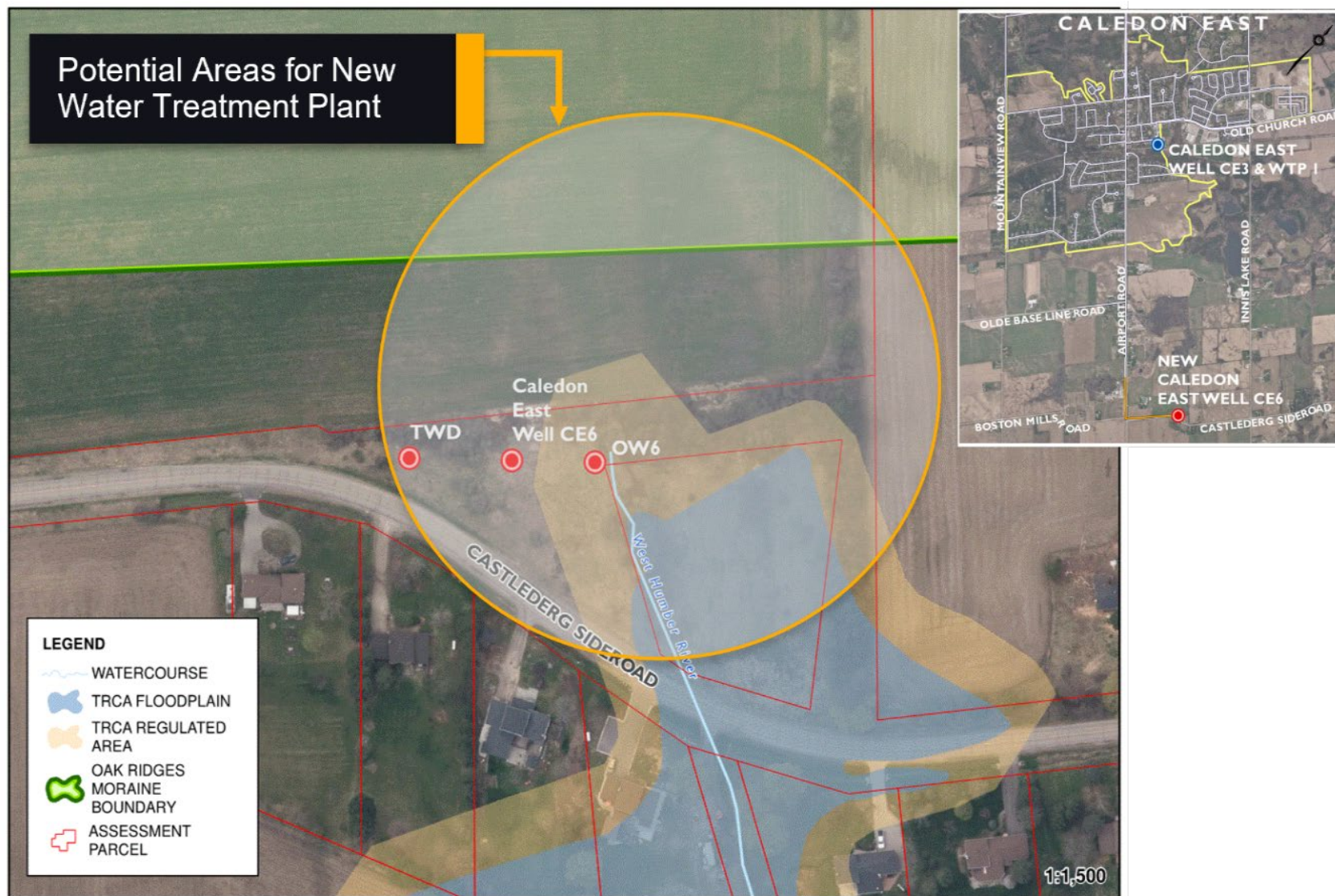
Figure 11: Potential Location for New Water Treatment Plant
