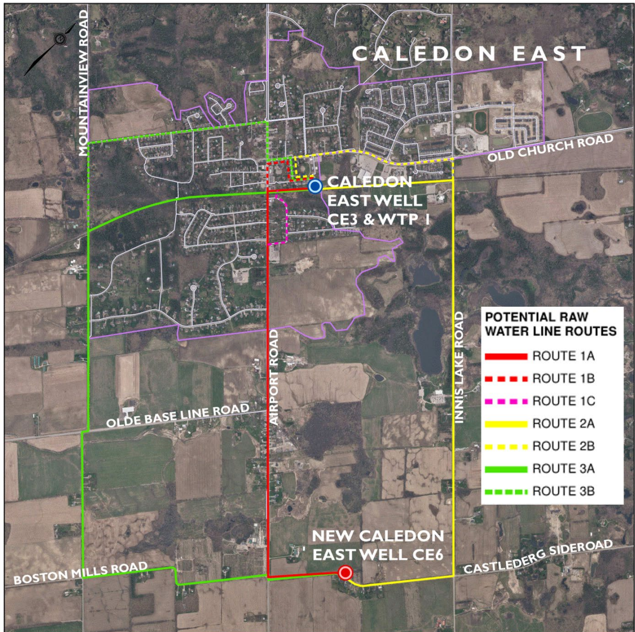
Figure (i): Option 1 – Obtain Additional Supply Capacity through a connection between New Well CE6 and Existing Caledon East Water Treatment Plant #1 (WTP1)
