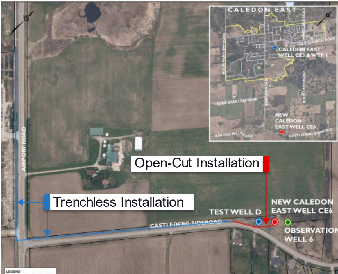
Figure (v): Preferred Feedermain Design Concept - Option F2 Pipe installation predominantly by trenchless methods with minimum open cut sections
