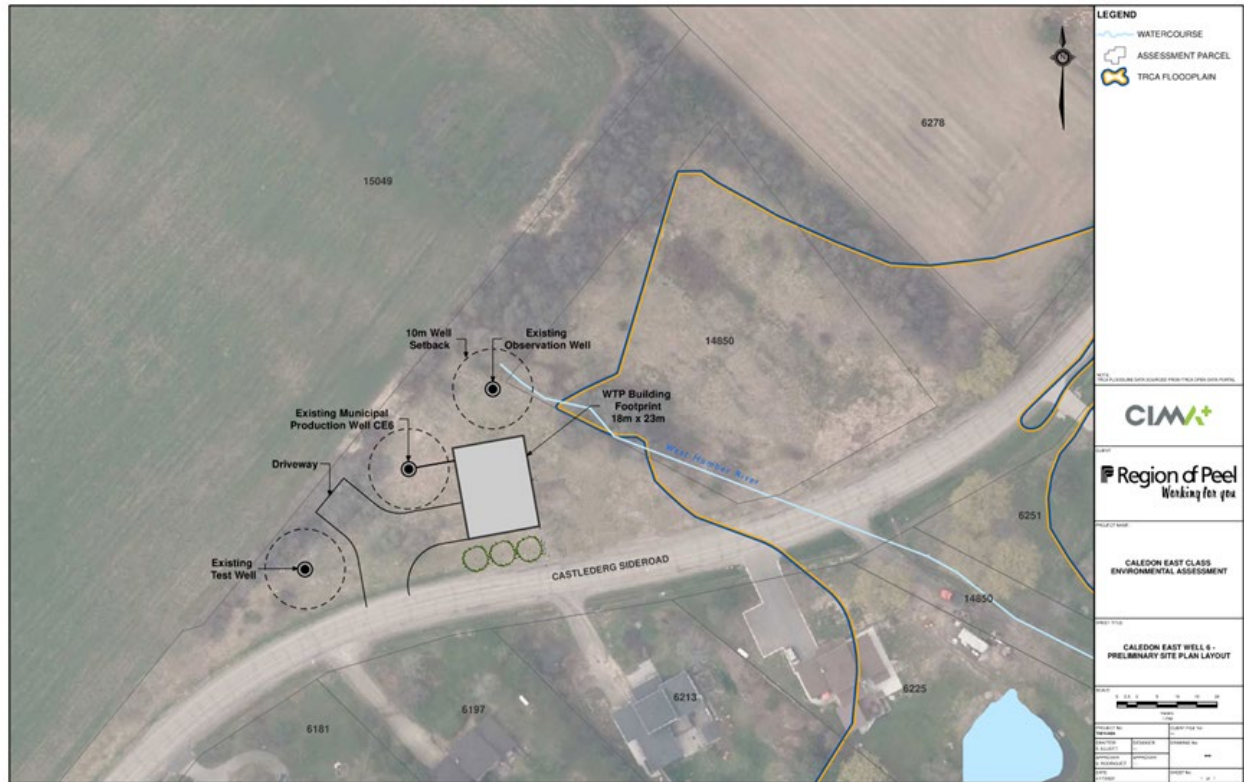
Figure (iii): Conceptual Site Plan – New Water Treatment Plant on CE6 well site
