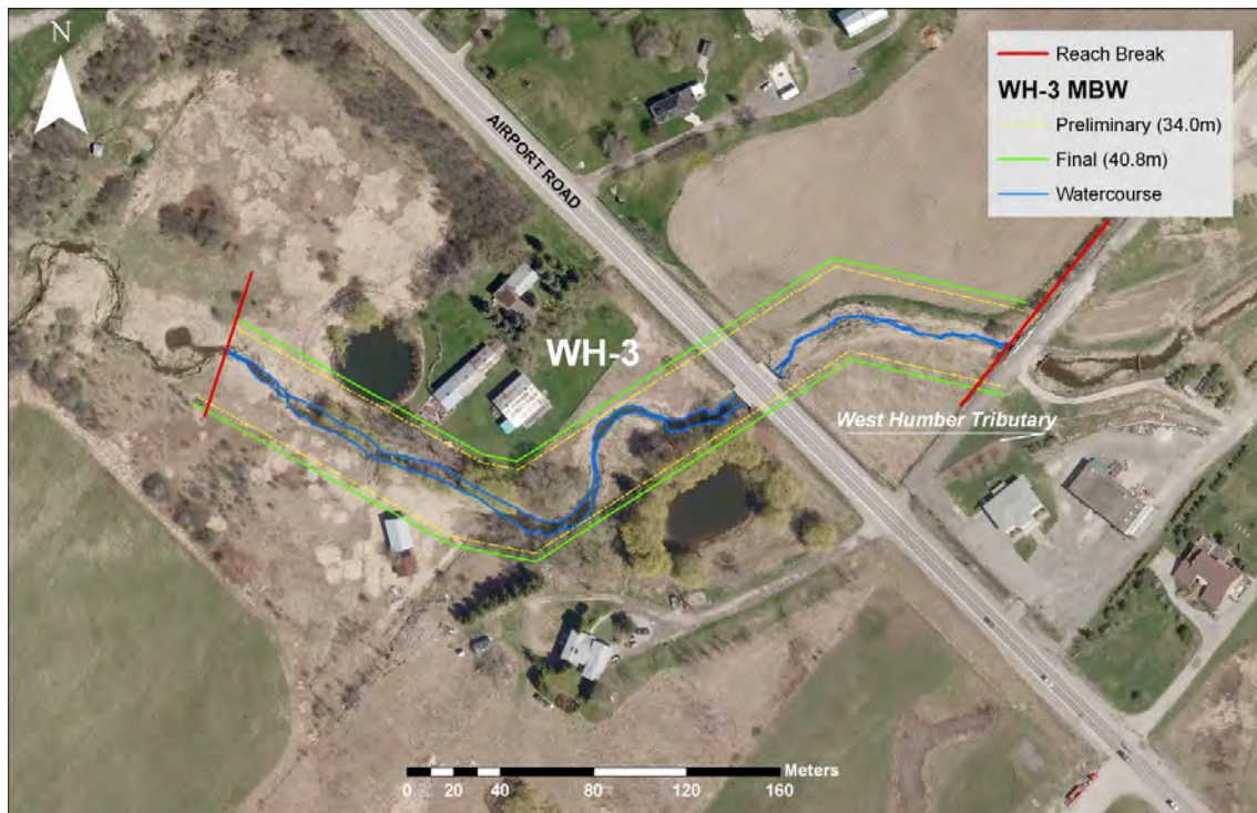
Figure 6.3: Delineation of preliminary meander belt width and factor of safety applied to West Humber Tributary reach WH-3.
