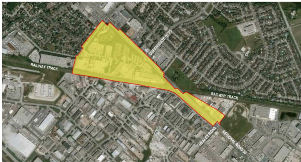
Figure 4.1: External Drainage Area That Contributes into Study Area
