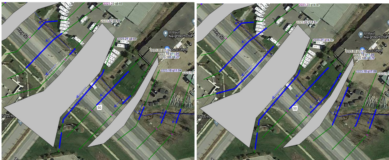
FIGURE 26 Culvert 5 and 6 – Water Extents on Cross-sections during the 25-Year (Left) and Regional Event (Right)
