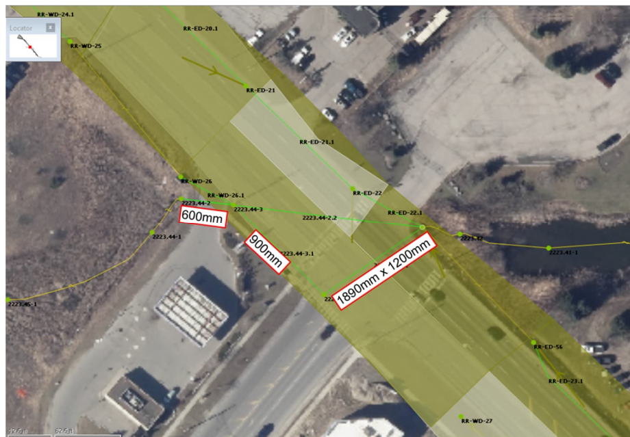
Figure 5. 1: George Bolton Parkway and -Highway 50 Intersection Culverts
