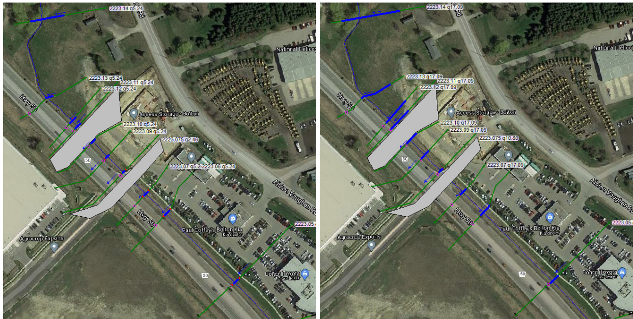
FIGURE 27 Culvert 7 and 8 – Water Extents on Cross-sections during the 2-Year (Left) and Regional Event (Right)
