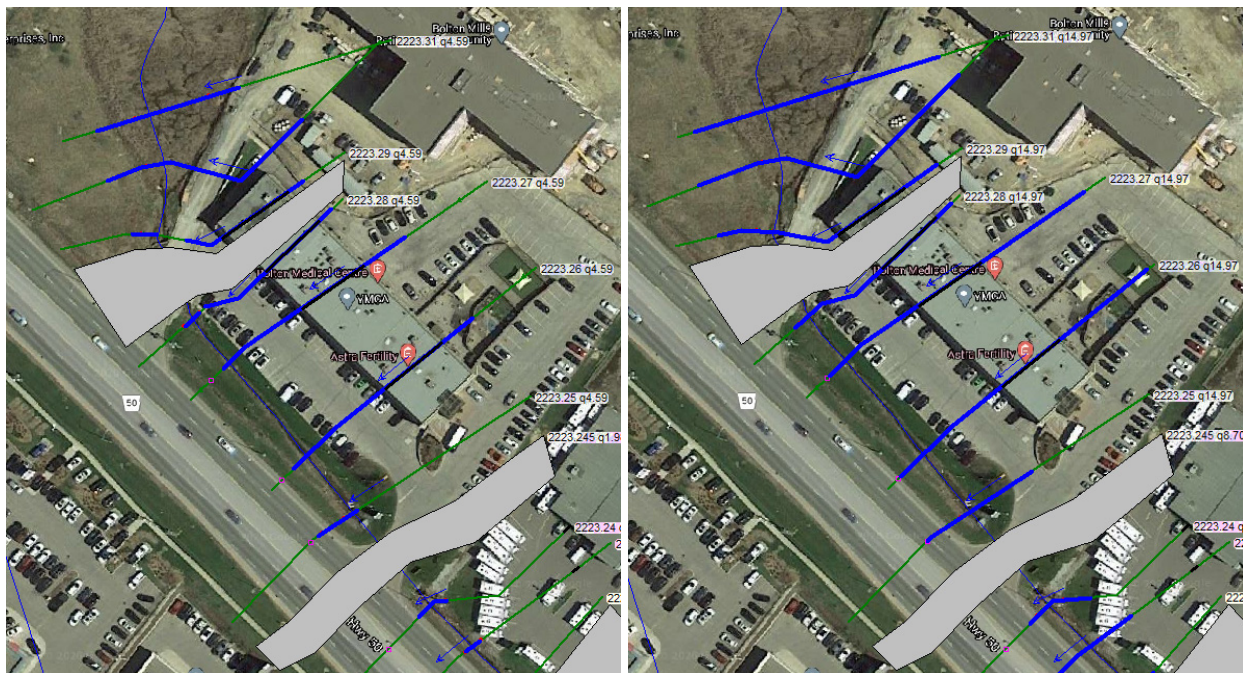
FIGURE 24 Culvert 3 and 4 – Water Extents on Cross-sections during the 2-Year (Left) and Regional Event (Right)
