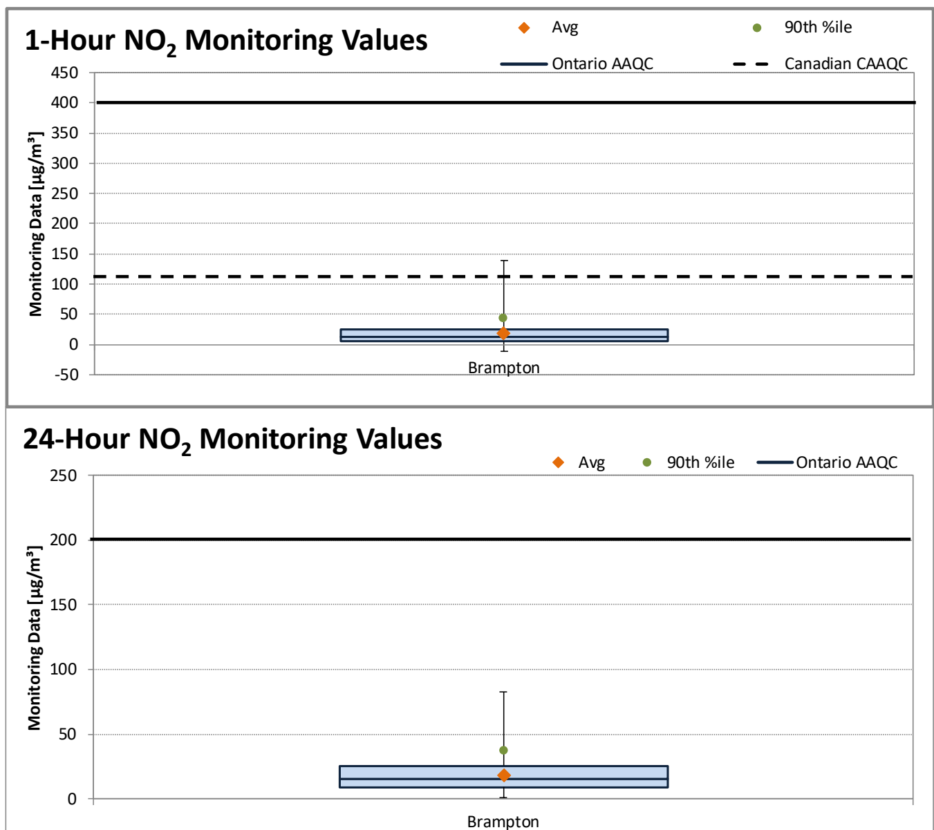
Figure 3: Measured 1-hour and 24-hour Nitrogen Dioxide (NO 2 ) Concentrations at the Brampton Station
