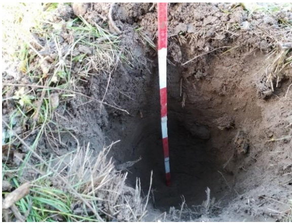
Image 9: Intact soil stratigraphy demonstrating topsoil (A-horizon) overlying subsoil (B-horizon).
