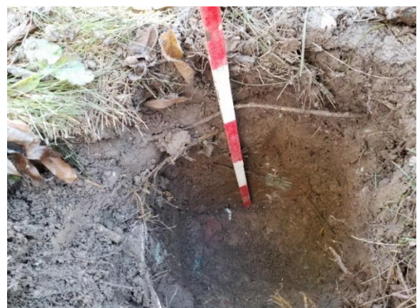
Image 12: Disturbed soil stratigraphy demonstrating redeposited topsoil overlying fill; intact topsoil (A-horizon) is absent.
