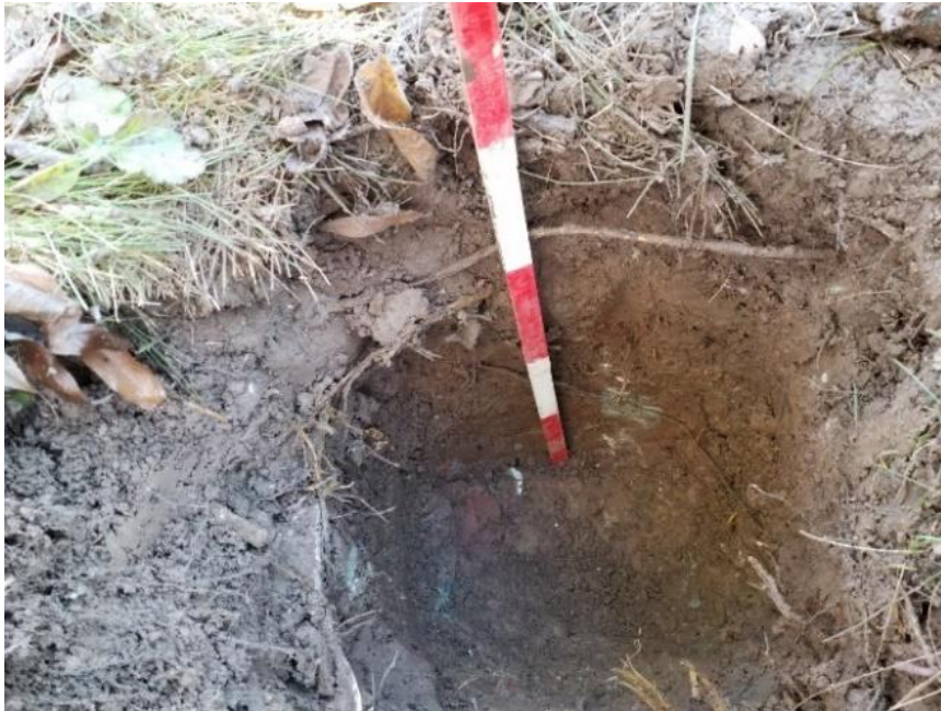
Image 21: Disturbed soil stratigraphy demonstrating redeposited topsoil overlying fill; intact topsoil (A-horizon) is absent
