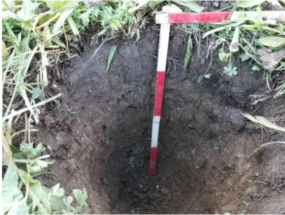
Image 13: Disturbed soil stratigraphy demonstrating redeposited topsoil overlying fill; intact topsoil (A-horizon) is absent.
