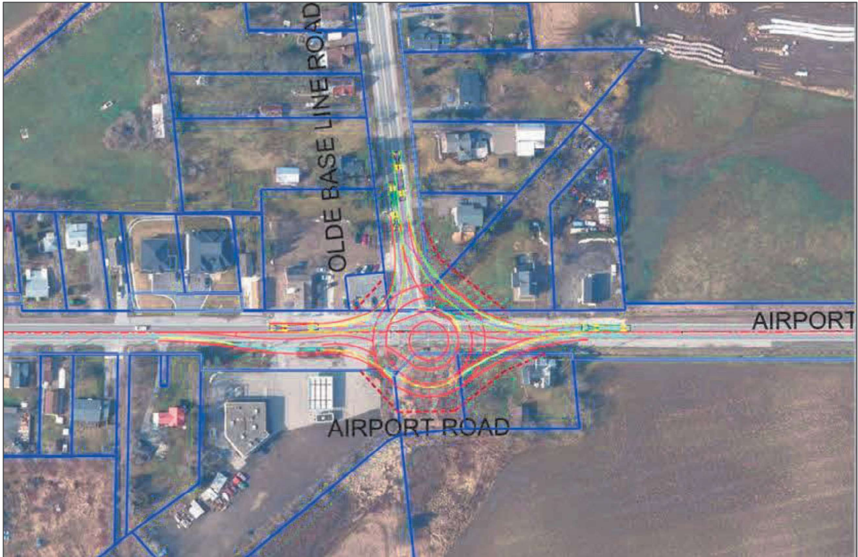
Exhibit 4-51: Roundabout Concept Plan for Airport Road & Olde Base Line Road (Not Carried Forward)
