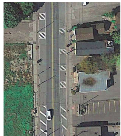
Exhibit 5-1 – Pavement Markings on Airport Road in Caledon East
