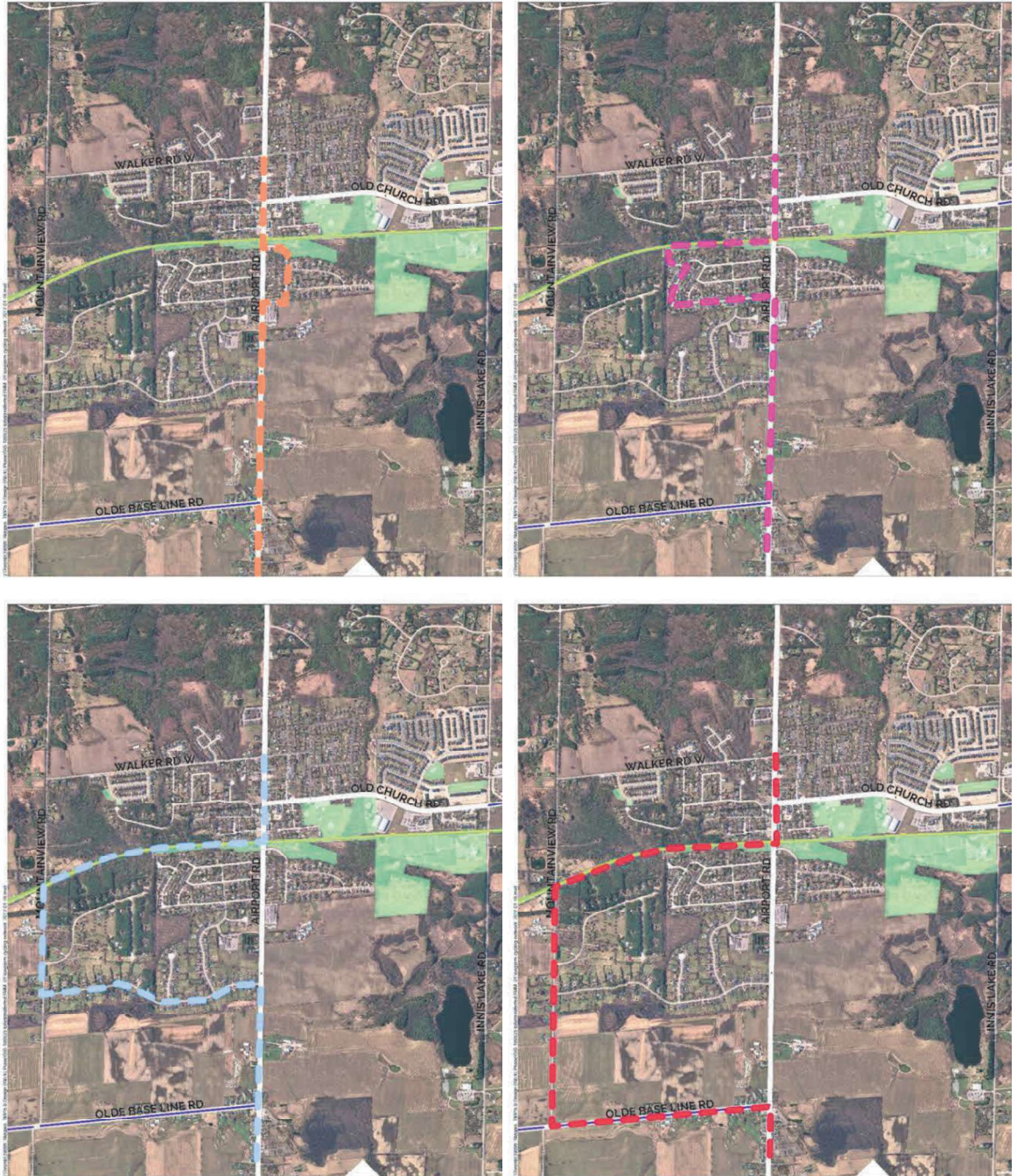
Exhibit 6-11: Potential Detour Routes along Airport Road from the Caledon Trailway Path to Hilltop Drive
