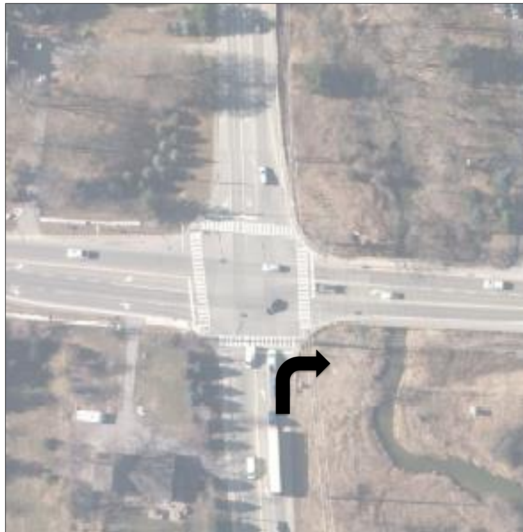
Alternative Solution #2 Additional Northbound Right Turn Lane
