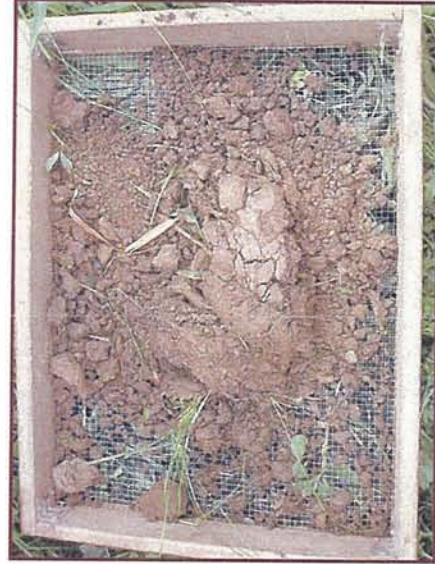
Figure 8-2: Mottled, Disturbed Soils Observed Along Alfalfa Field, East Side of Dixie Road in Section 3
