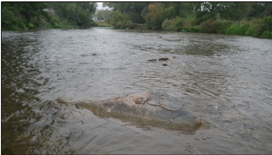
6. Downstream of Credit River Bridge – large boulder with downstream scour depth of 0.57 m.
