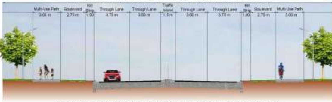
Clarkway Drive South of 'Main Street' - 36.0 m Right-of-Way, No Median, Cycling and Sidewalks
