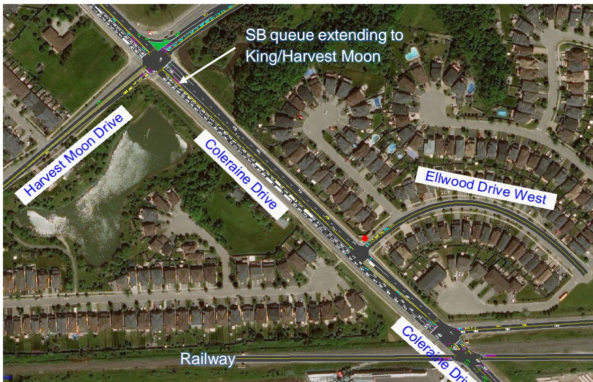
Figure 23 – 2041 AM Southbound Queues During Train Crossing
