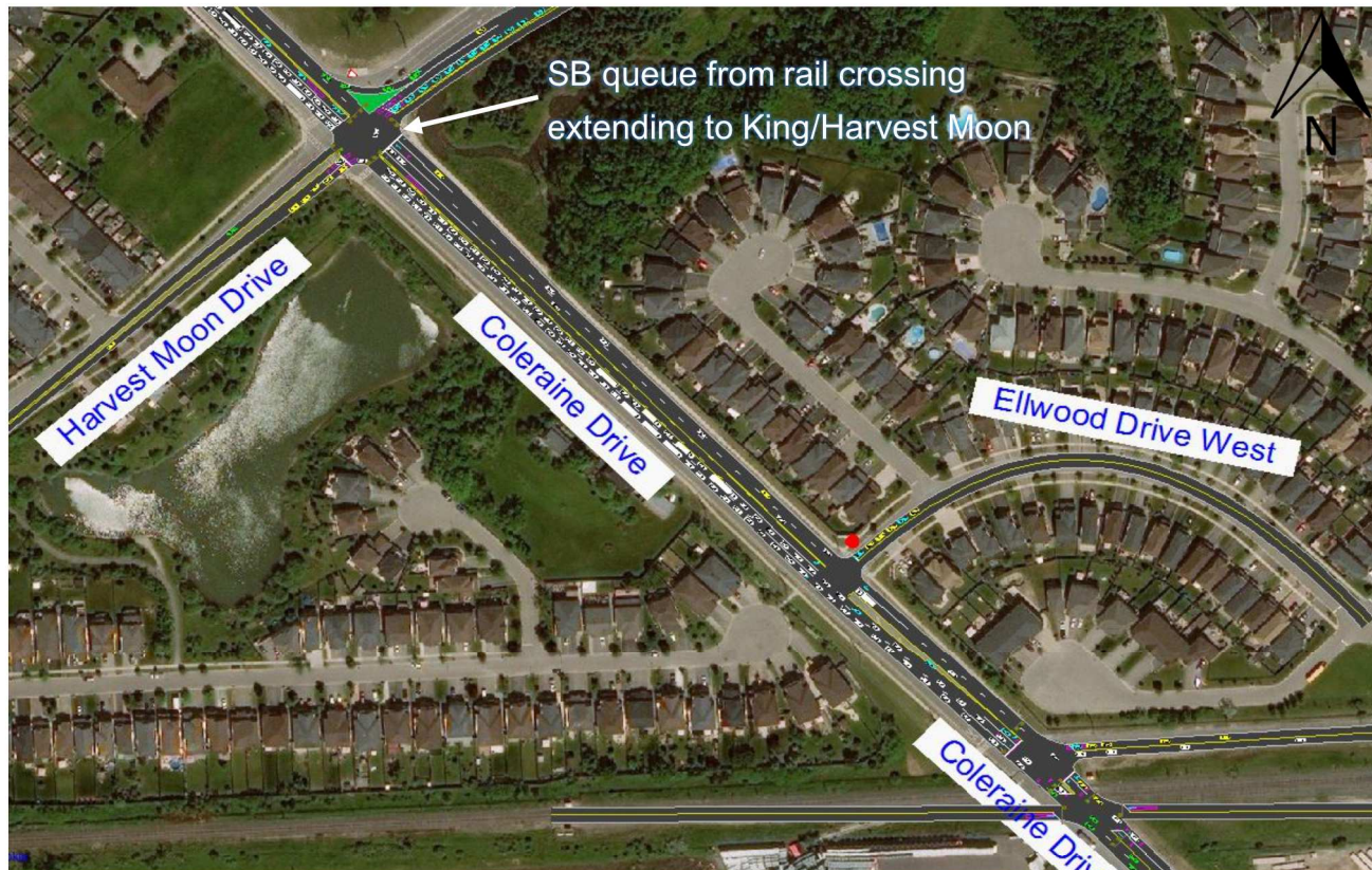
2041 AM Southbound Queues During Train Crossing
