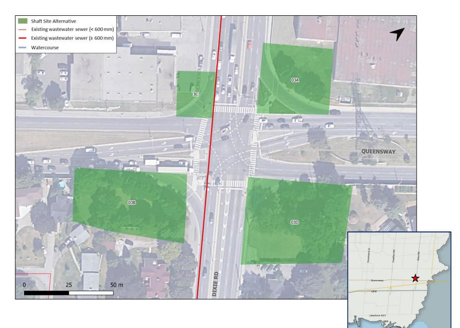
**Shaft 6** is required to support constructability of the tunnelled alignment along Queensway East and Cawthra Road as well as to connect into the proposed trunk sewer along Cawthra Road. This connection is required to support the overall strategy for diverting flows and increasing capacity within the system. Three alternatives were selected for evaluation.
