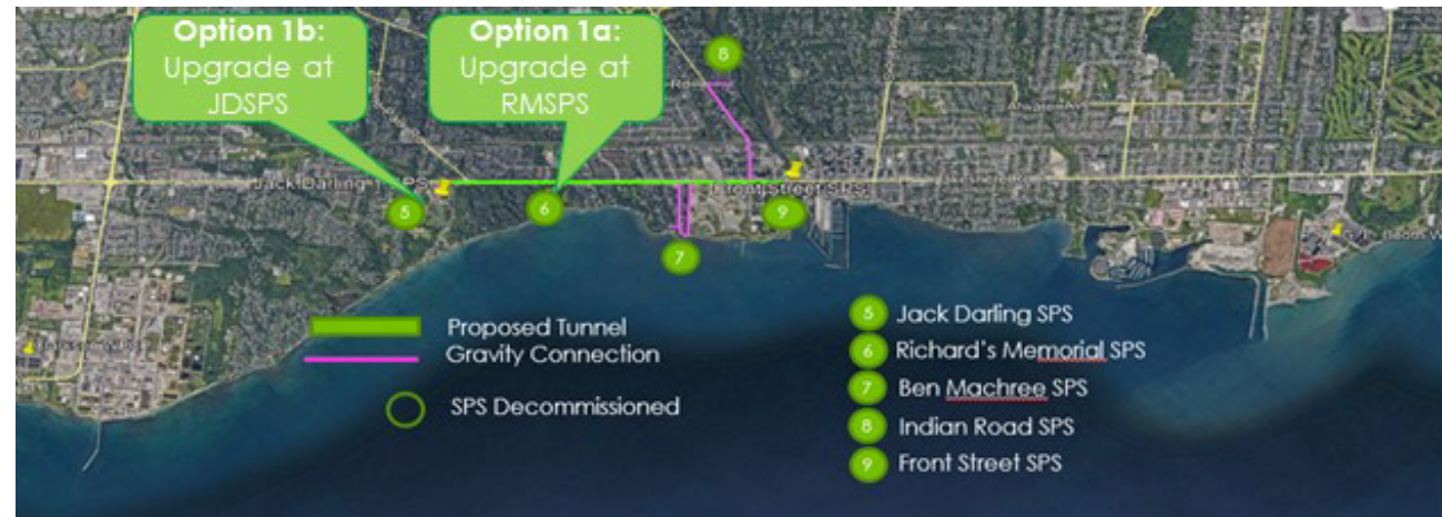
Option 1: Tunnel Entirely within Rock and Within Current Limits of EA (Upgrade at RMSPS or JDSPS)
