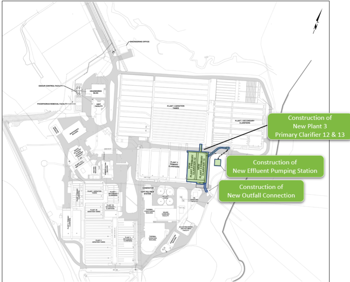
Figure 4 Plant 3 Primary Clarifier Capacity Recovery Site Plan
