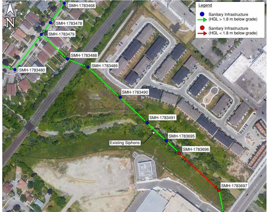
Figure 12: Location of Sanitary Infrastructure with HGL < 1.8 m below Grade – 25 Year SCS Storm (Existing Sewer Routing)
