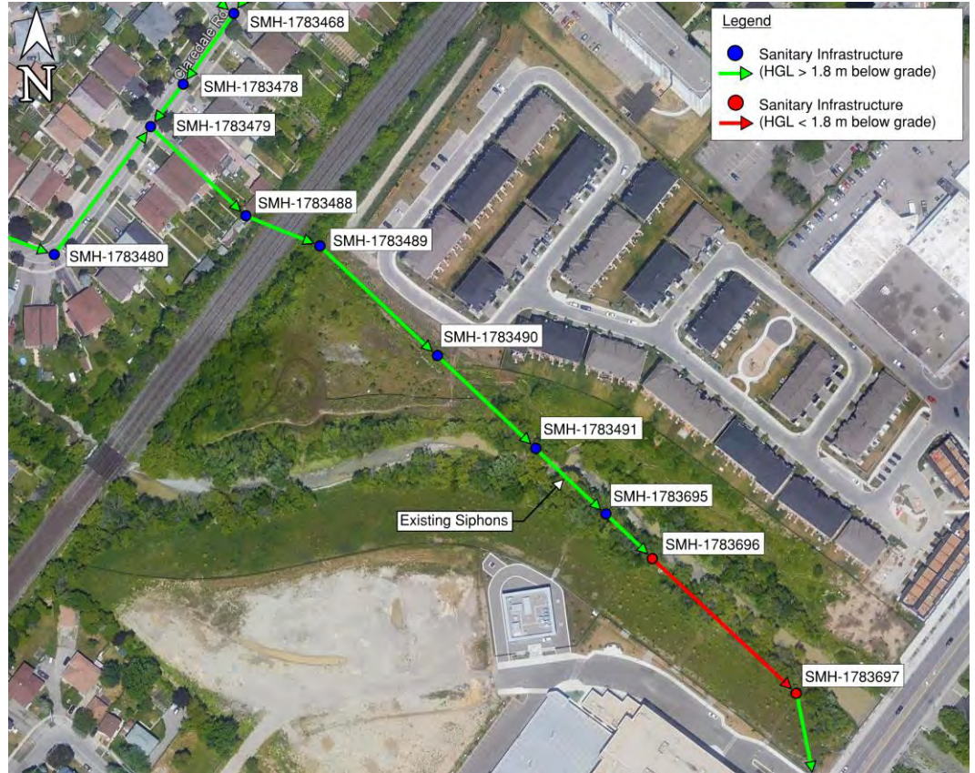
Figure 9: Location of Sanitary Infrastructure with HGL < 1.8 m below Grade – 5 Year SCS Storm (Existing Sewer Routing)
