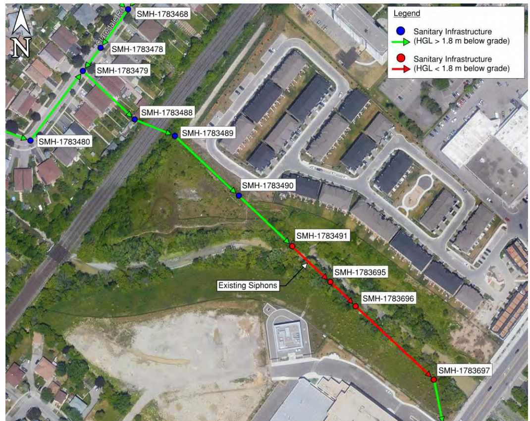
Figure 15: Location of Sanitary Infrastructure with HGL < 1.8 m below Grade – 100 Year SCS Storm (Existing Sewer Routing)
