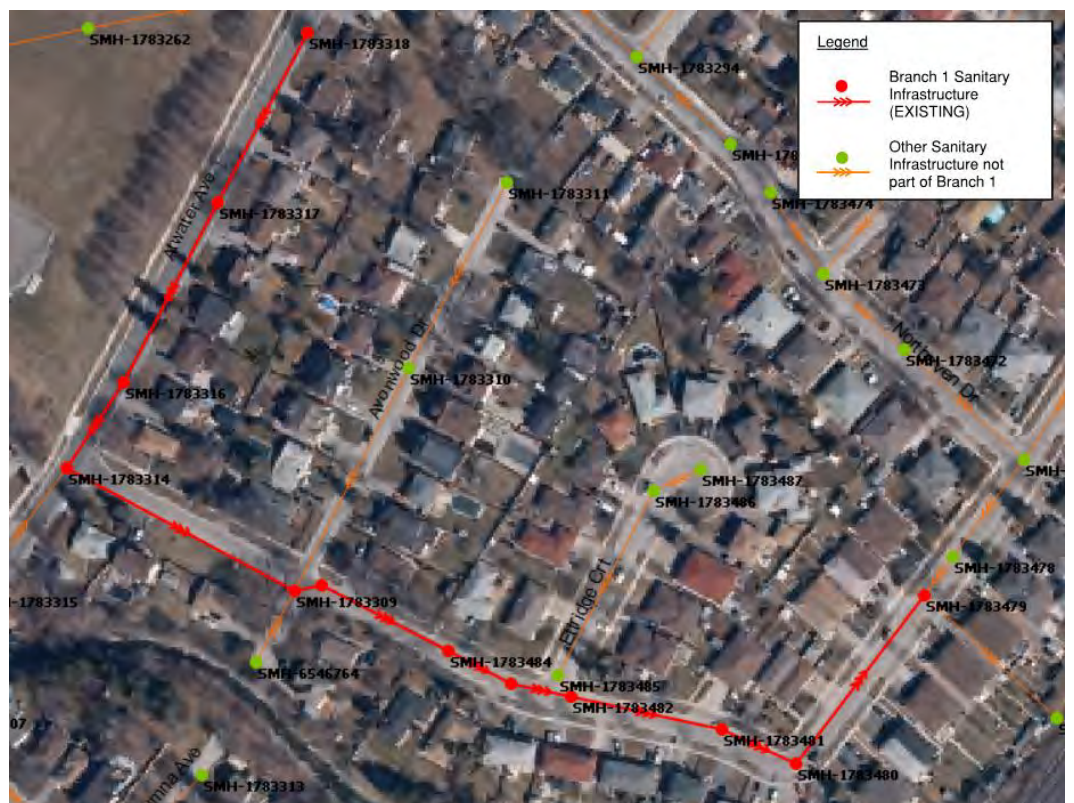
Figure 4: Claredale Road Sanitary Catchment Area – Branch 1
