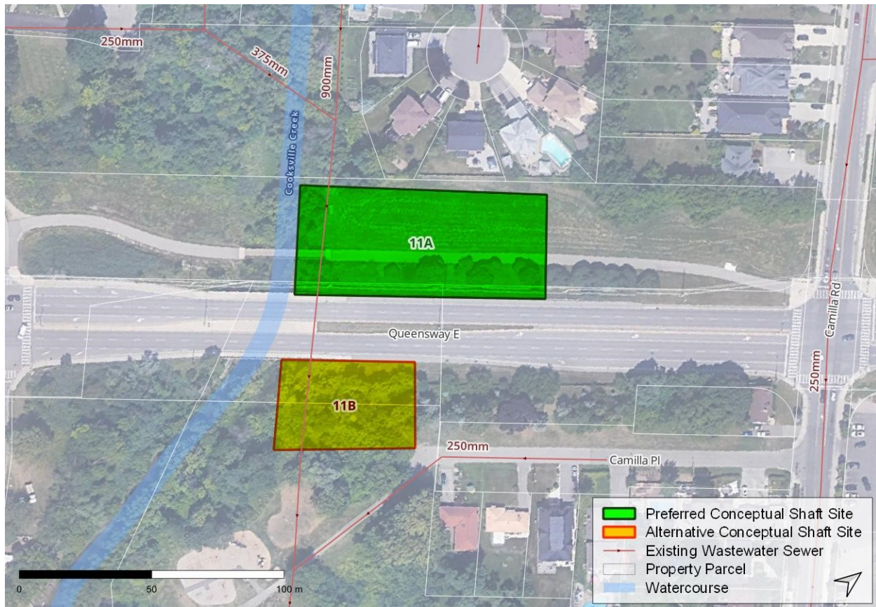
Figure 32: Conceptual Shaft 11 Alternatives
