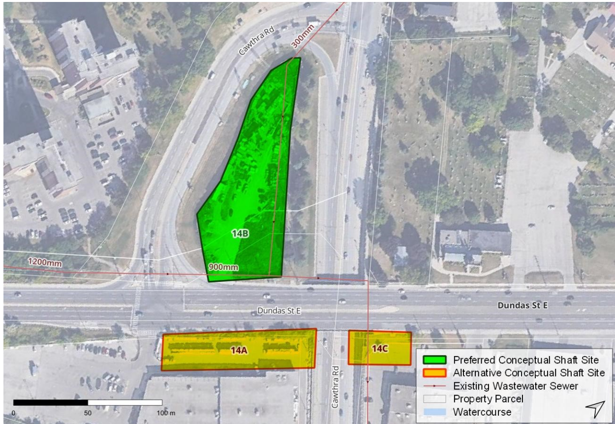
Figure 34: Conceptual Shaft 14 Alternatives
