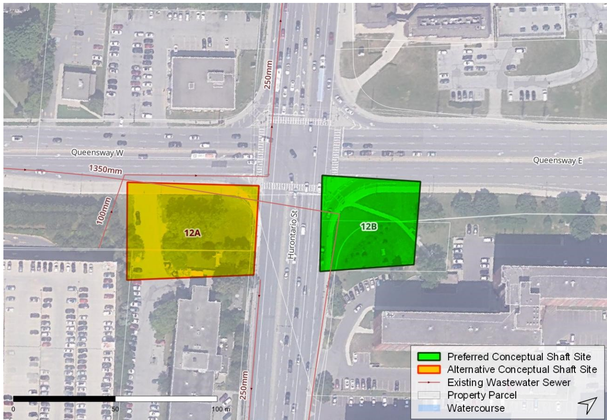
Figure 33: Conceptual Shaft 12 Alternatives
