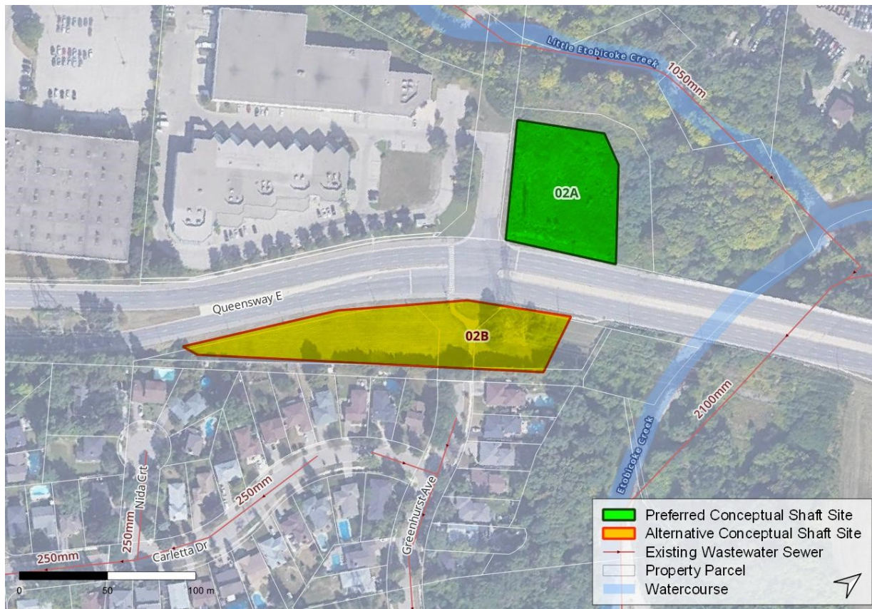
Figure 26: Conceptual Shaft 2 Alternatives
