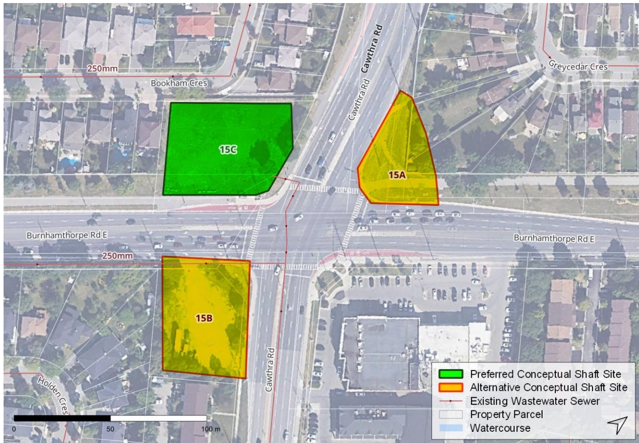
Figure 35: Conceptual Shaft 15 Alternatives
