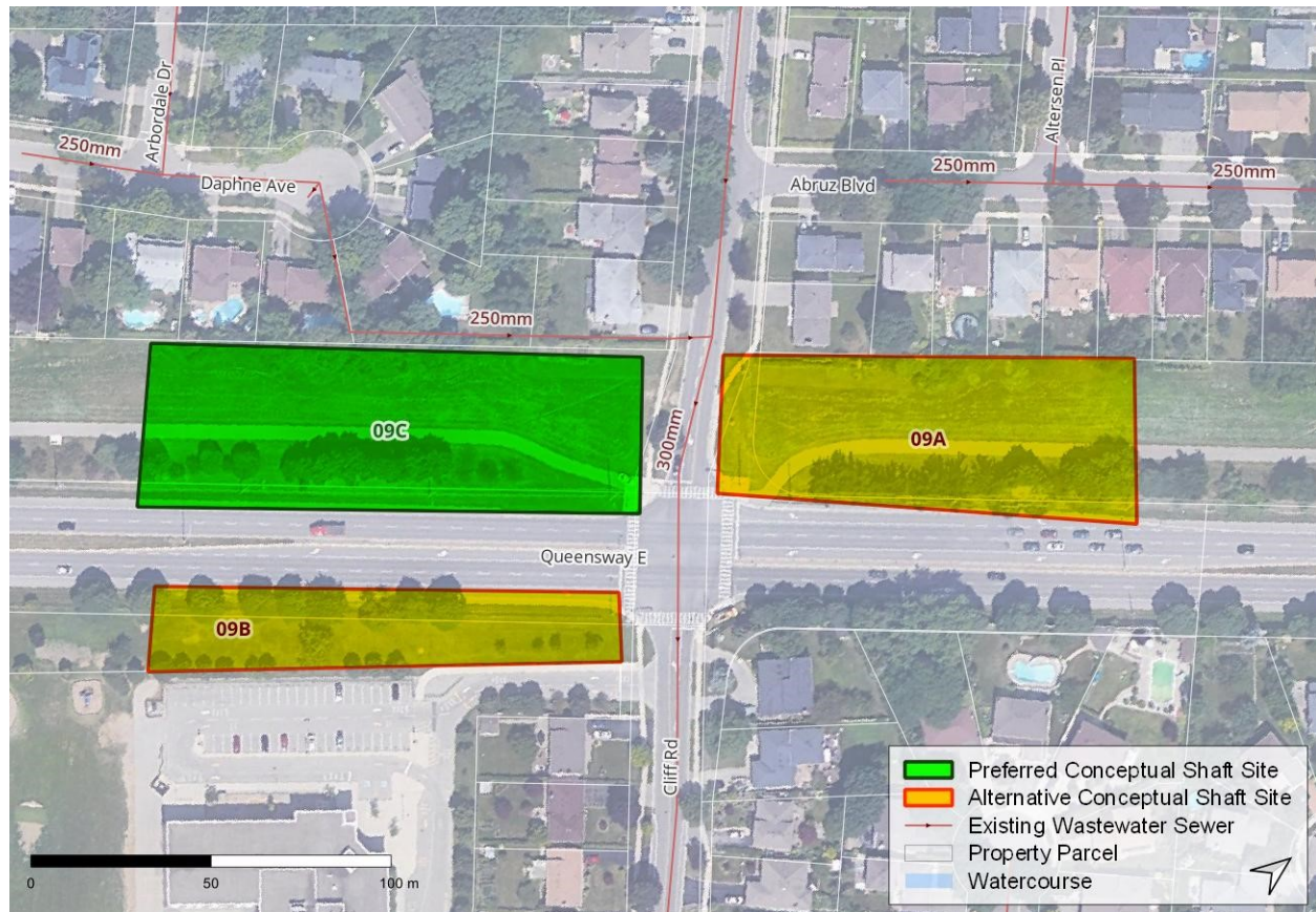
Figure 31: Conceptual Shaft 9 Alternatives
