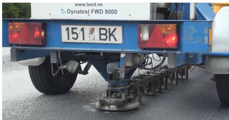
c - Falling Weight Deflectometer Testing (Load Cells and Geophones)
