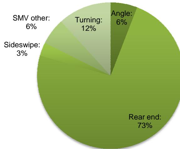
Furthermore, the right-most (third) southbound lane on Cawthra Road exits to the eastbound QEW immediately upstream of the traffic signal, resulting in this lane maintaining high speeds while the left two lanes serve as queue storage. The differential in speed across the three southbound lanes may be a contributing factor to the prevalence of rear-end collisions on the approach to this intersection.
