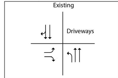
The **Dundas Ramp** intersection operates at LOS C during the AM and PM peak hours. The intersection operates under split phasing for east-west movements (given the low demand on the east leg). The safety analysis at the Dundas Ramp indicates a clear trend of rear-end collisions immediately south of the ramp. The safety analysis also indicates that NBL turn vehicles may be misjudging gaps in southbound traffic likely due to high speeds.
