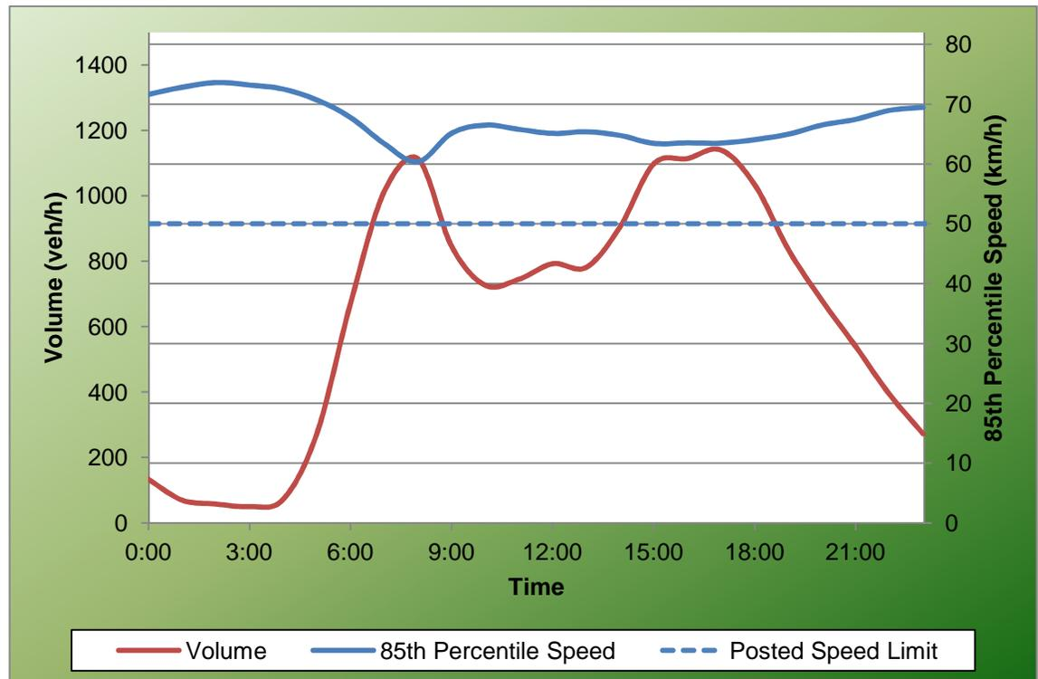
It can be seen that speeds well above the 50 km/h posted limit are maintained throughout the day, with the most excessive speeds in the overnight hours reaching well over 70 km/h.
