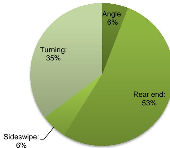
The collision frequency (3.4 per year) and collision rate (0.28 collisions per million intersecting vehicles) are among the lowest of signalized intersections within the Cawthra Road corridor, with a typical pattern of collisions observed.
