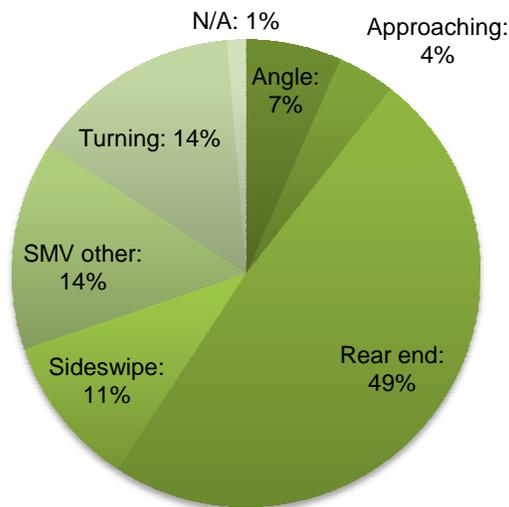
There was also a relatively high prevalence of single motor vehicle (SMV) collisions caused by loss of control on the eastbound and westbound approaches to this intersection. Much like the North Service Road, these approaches have sharp bends as illustrated in the collision diagram in **Appendix A**. Given that almost all of the loss-of-control collisions at this intersection occurred in wet, snowy or otherwise inclement weather conditions, it should be investigated how the
