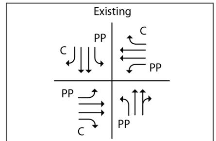
The **Silver Creek** intersection operates at LOS C during the AM and PM peak hours. It is a three-leg intersection. There are two driveways on the east side, at the intersection. To access properties on eastside, a southbound left is available; however does not affect signal phasing. The northbound left is heavy during the PM peak and exceeds 350 veh/hr.
