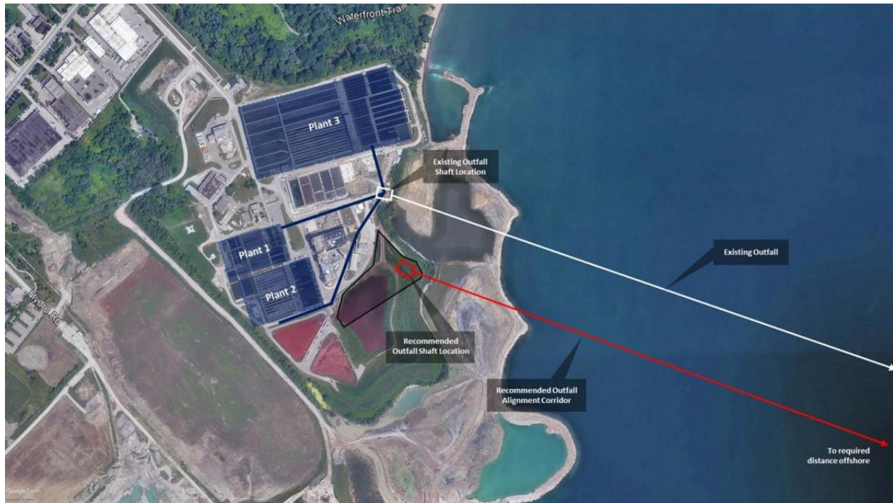
Figure 5-1: Recommended Outfall Layout
