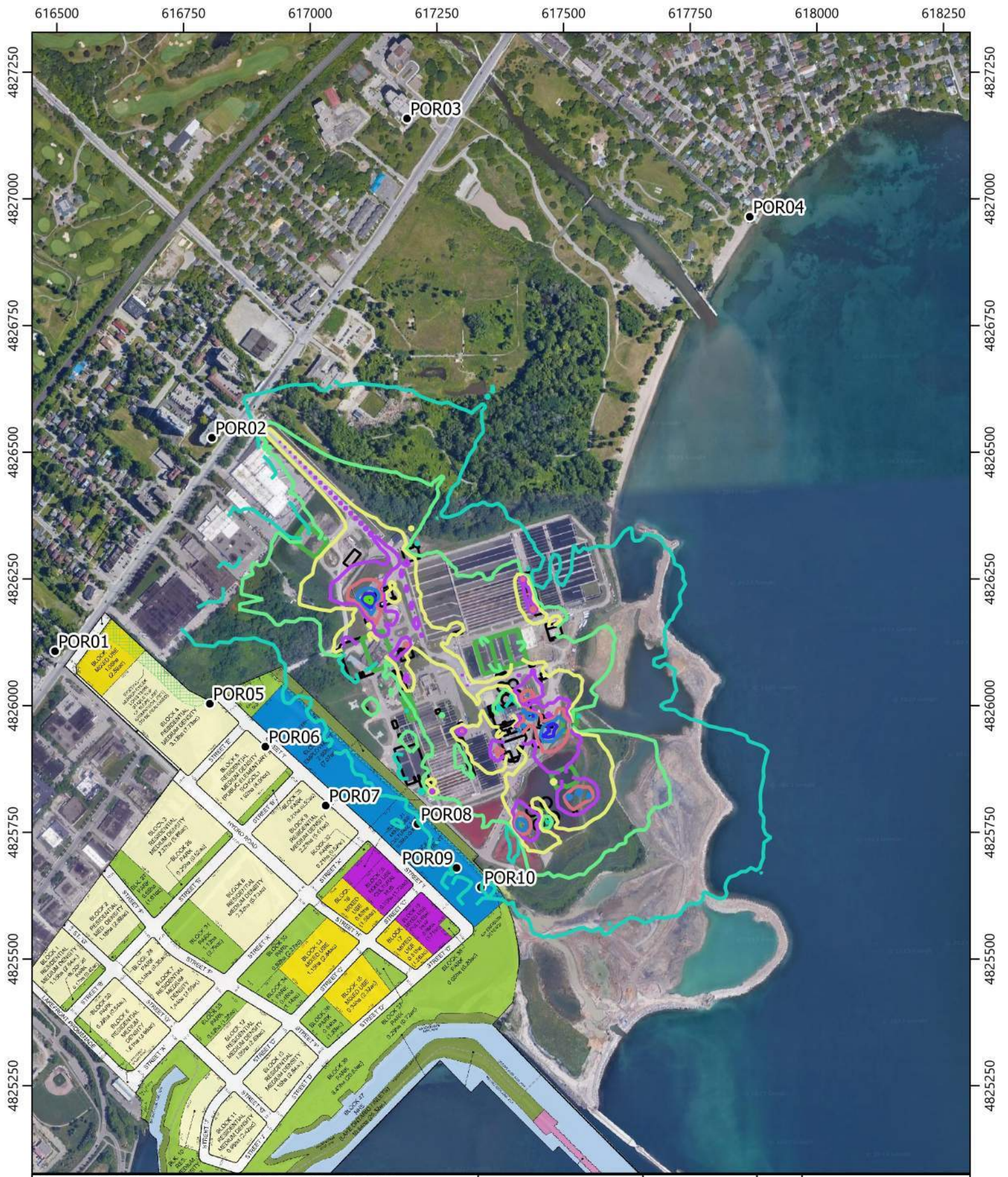
Figure 9: Noise Contours for Future Predictable Worst-Case Operations - Daytime/Evening Acoustical Assessment Report: G.E. Booth WWTP 1300 Lakeshore Rd E, Mississauga ON P.No. CA02694 Date: 09/2023 50 dBA 60 dBA 70 dBA 55 dBA 65 dBA
