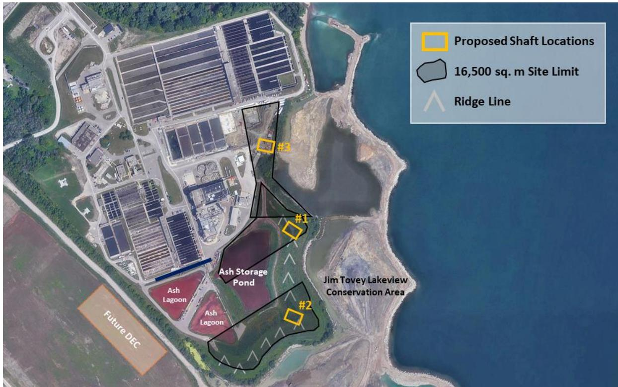
Figure 8-12 Alternative Outfall Shaft Locations and Staging Areas
