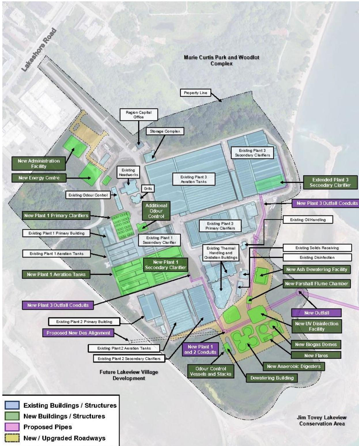
Figure 9-1 G.E. Booth WRRF Design Components
