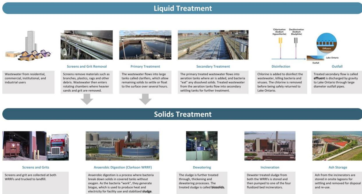
**Figure 5-4 G.E Booth WRRF Simplified Process Flow Diagram**
