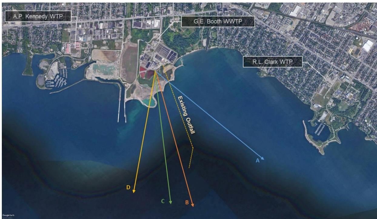
**Figure 8-14 Outfall Alignment Alternatives**
