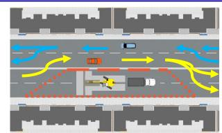
Stage 3: Surface works for the roadway will be done for one half of the road at a time. Surface work for the sidewalk / boulevard will be completed at the same time as the roadworks.
