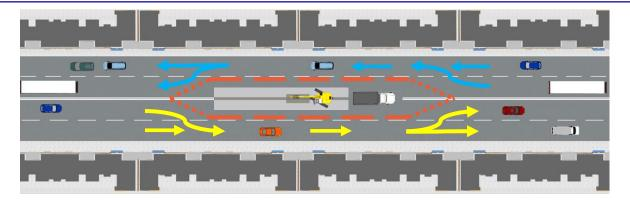
Stage 2: Installation of watermain and sewer connections to the houses and businesses on each side of the street.
