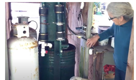
Jane explains how gas from her anaerobic digester is purified and compressed.
