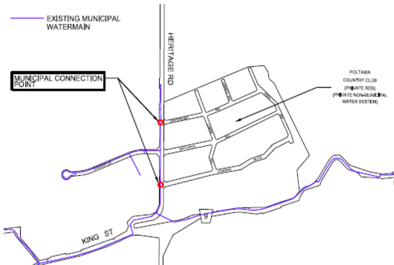
Figure 3: Poltawa Water Distribution System
