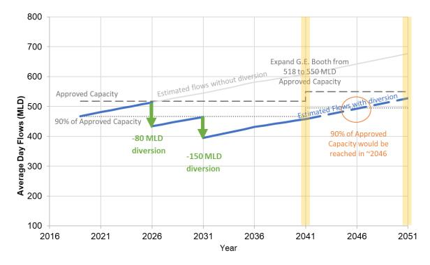
Figure E-3: Preferred Solution: Diversion and Expansion Approach for the G.E. Booth WRRF
