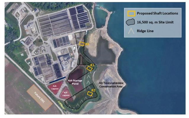
Figure E-4: Alternative Outfall Shaft Locations and Staging Areas
