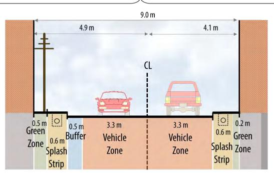
Constrained Rural Main Street (9.0 m Typical ROW – Minimal Paved Buffer on Both Sides and Minimal Green Zone)
