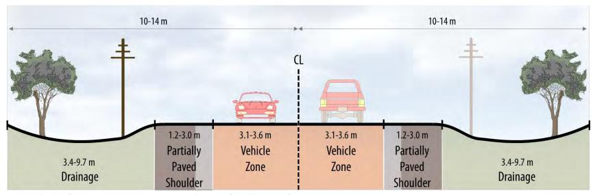
Note: Total right-of-way is predominantly 20-23 m; paved portion of shoulder ranges from 0-1.0 m; majority of above ground utilities run on east side of the road and crosses over between sides
