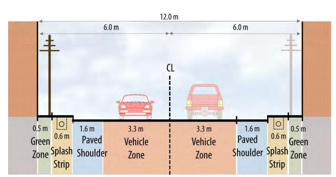
Constrained Rural Main Street (12 m Typical ROW – Sidewalk on Both Sides)
