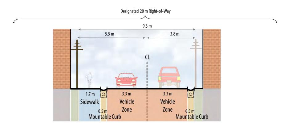
Constrained Rural Main Street (9.3 m Platform with Paved Shoulder on one side and Mountable Curb)
