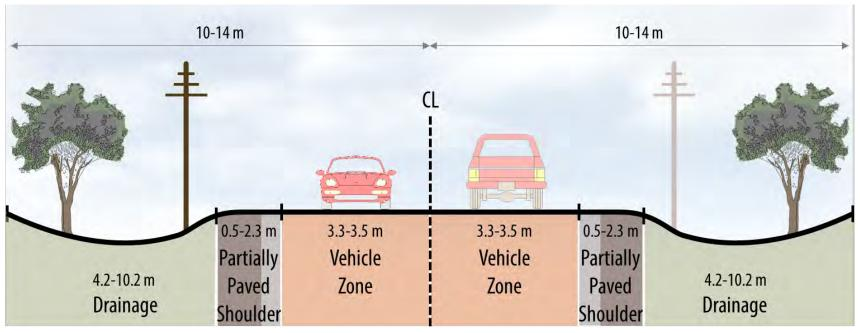
Note: Total right-of-way is predominantly 20 m; paved portion of shoulder ranges from 0-2.3 m; majority of above ground utilities run on one side of the road and crosses over between sides
