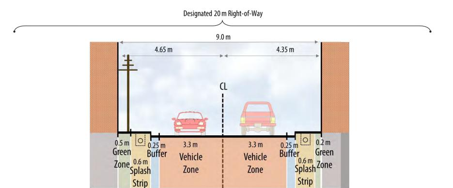
Constrained Rural Main Street (8.0 m Platform – Narrow Paved Shoulder on Both Sudes, Existing Splash Strip on One Side and No Green Zone)
