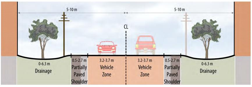
Note: Total right-of-way is predominantly 20 m; paved portion of shoulder ranges from 0.2-2.0 m; majority of above ground utilities run on one side of the road and cross over between sides
