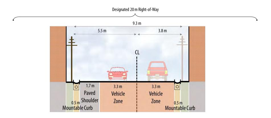
Constrained Rural Main Street (10.5m Typical ROW – Narrow Paved Buffer on Both Sides)
