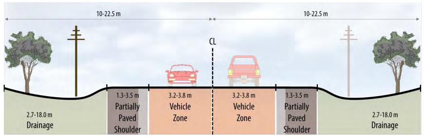
Note: Total right-of-way is predominantly 30 m; paved portion of shoulder ranges from 0.2-1.5 m; majority of above ground utilities run on north side of the road and crosses over between sides
