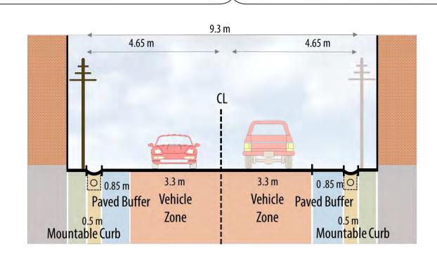
Constrained Rural Main Street (9.0 m Typical ROW – Narrow Paved Buffer on One Side and Minimal Green Zone)
