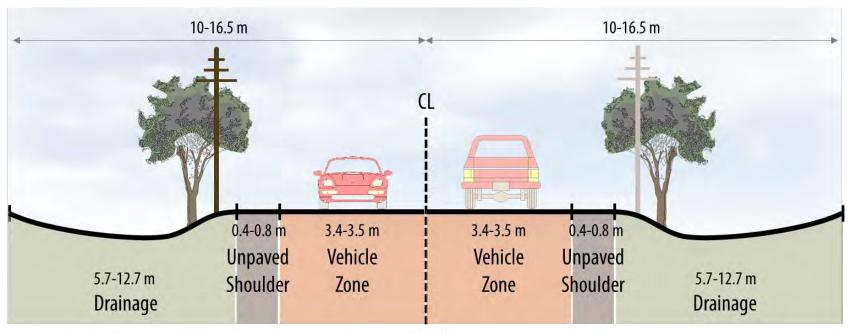
Note: Total right-of-way is predominantly 20-25 m; no paved portion of shoulder exists; majority of above ground utilities run on one side of the road and cross over between sides
