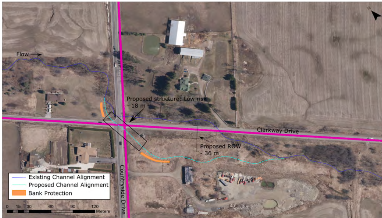
FIGURE 8b Clarkway Tributary Crossing Countryside Drive and Clarkway Drive (Crossings D and E) - Alignment Option 2
